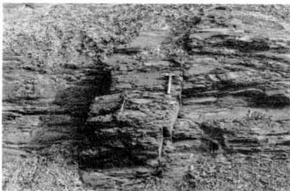
Figure 3. Planar fractures or joints developed in the Mahantango Formation. Groundwater occurs in secondary openings along fractures and bedding-plane separations in the bedrock aquifers.
