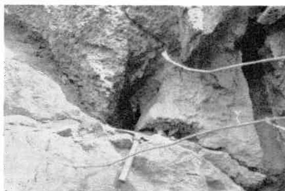
Figure 4. Solution openings in the Keyser Formation. Development of solution openings, primarily along fractures and bedding-plane separations, greatly increases the secondary permeability of carbonate rock.
