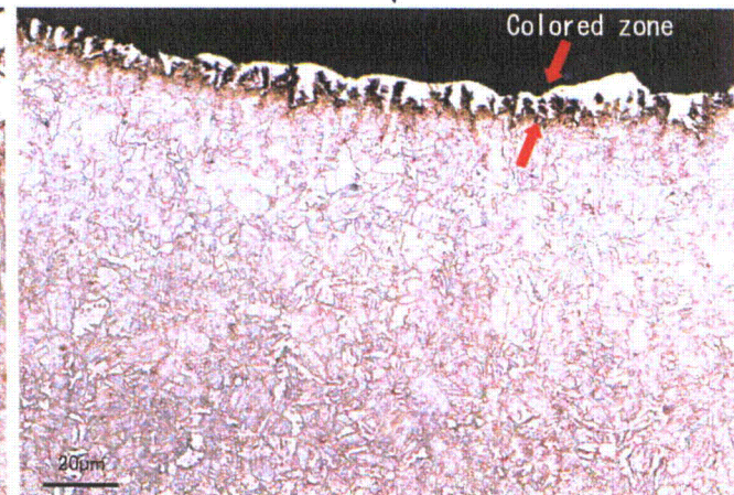
Figure A.48(1) Macro structure and micro structure of cross section of sample F
