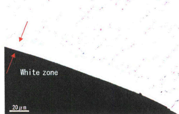
Fig.A.39(2) Microstructure observation of cross section of sample D (152 buttering and boundary between 152 buttering and stainless steel clad)
