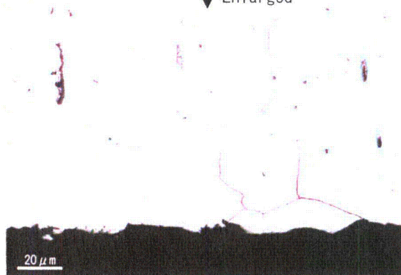
Fig.A.39(3) Microstructure observation of cross section of sample D (Stainless steel clad by ESW)
