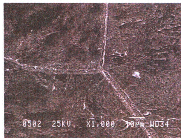
Fig. A. 20(2) SEM observation of fracture surface of sample B (152 buttering) (continued)
