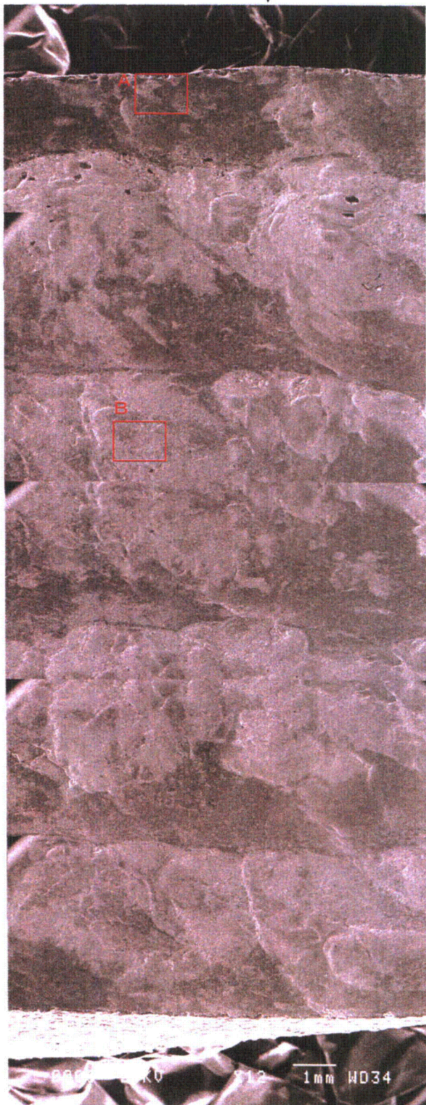
Fig. A. 21(1) SEM observation of fracture surface of sample B (Low alloy steel channel head)
