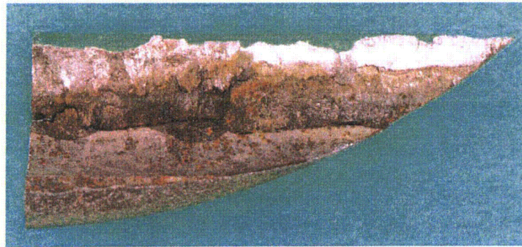
Fracture surface (from Direction C)
