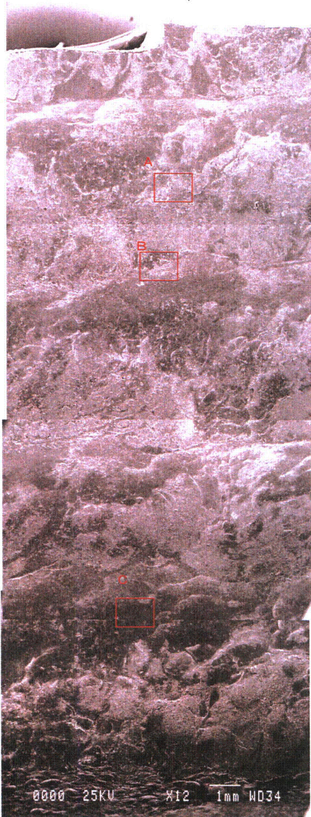
Fig. A. 20(1) SEM observation of fracture surface of sample B (152 buttering)
