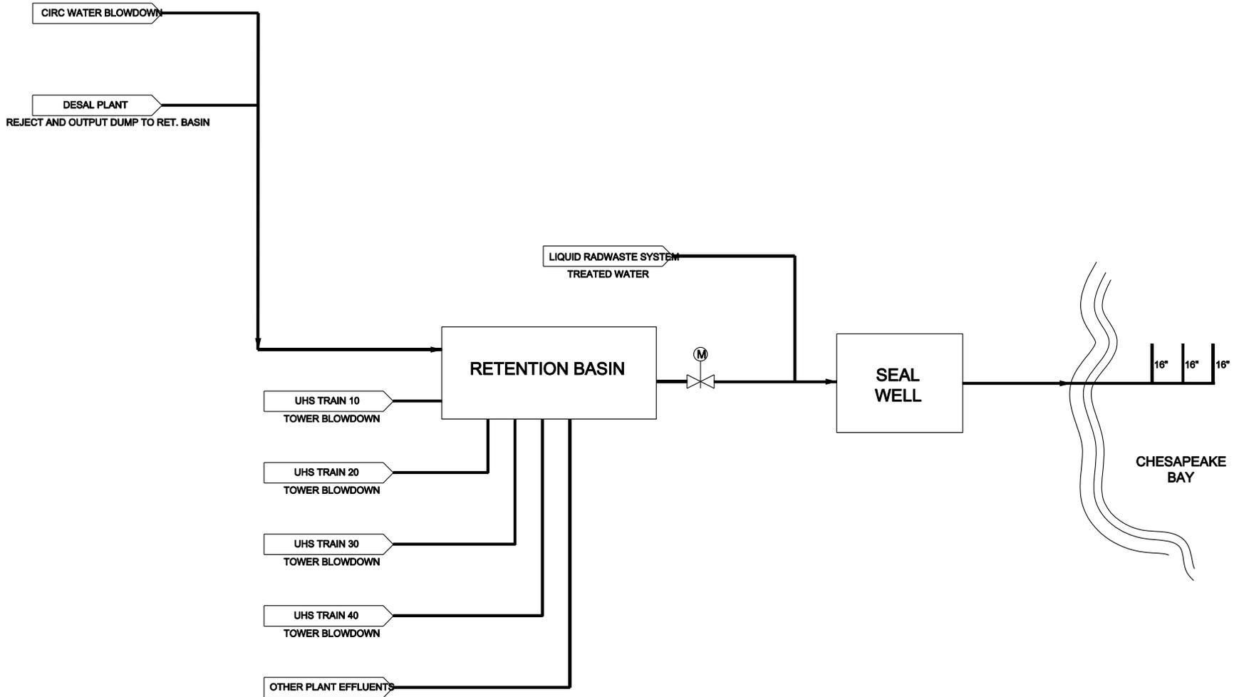
Figure 10.4-7—{Circulating Water System Plant Discharge}
