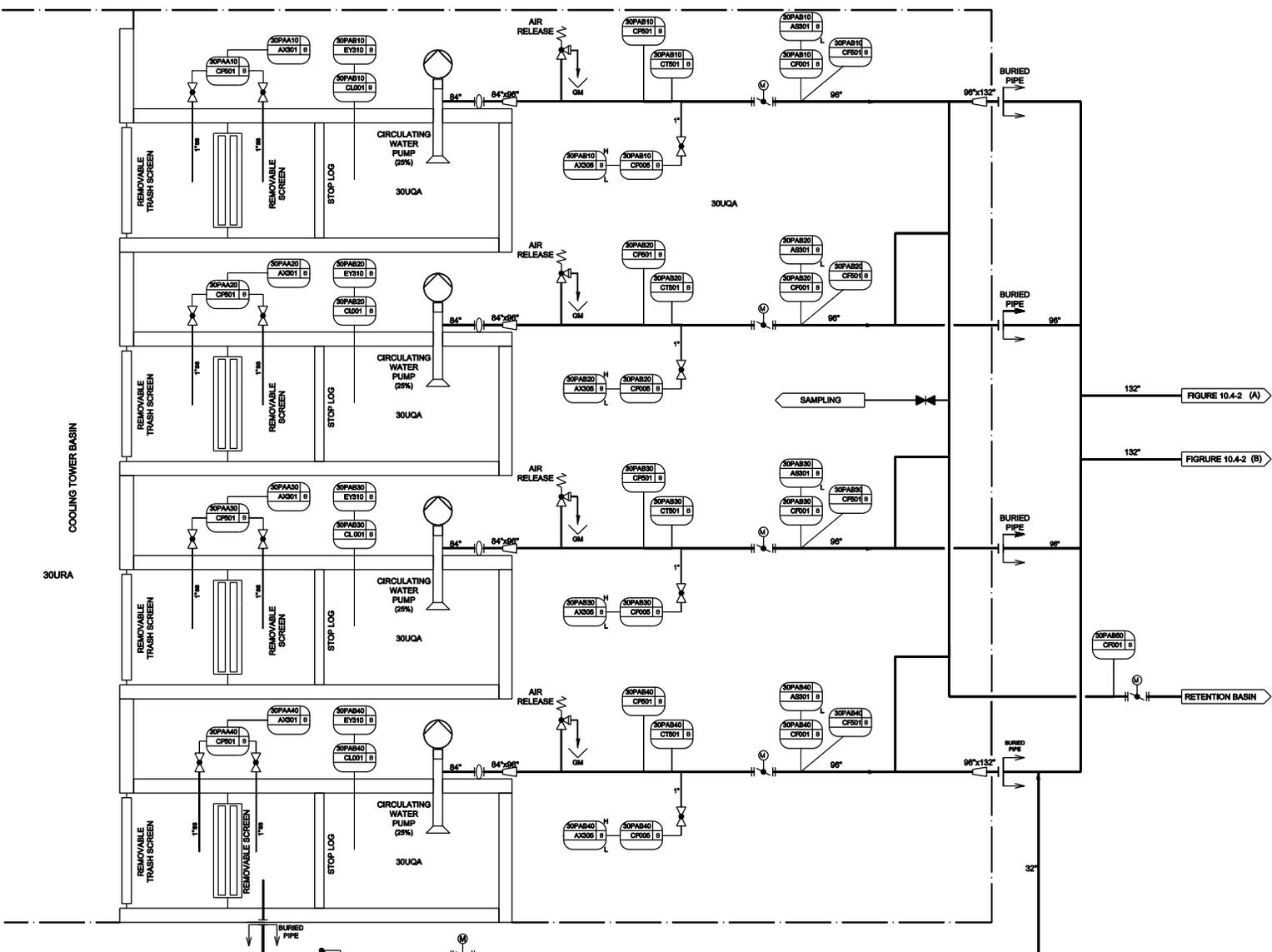
Figure 10.4-2—{Circulating Water System P & ID (Turbine Building)}
