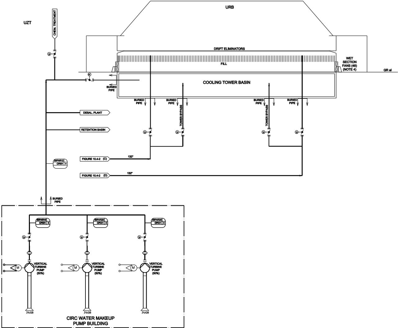
Figure 10.4-4—{Circulating Water System Makeup Pump Intake Structure (Plan View)}
