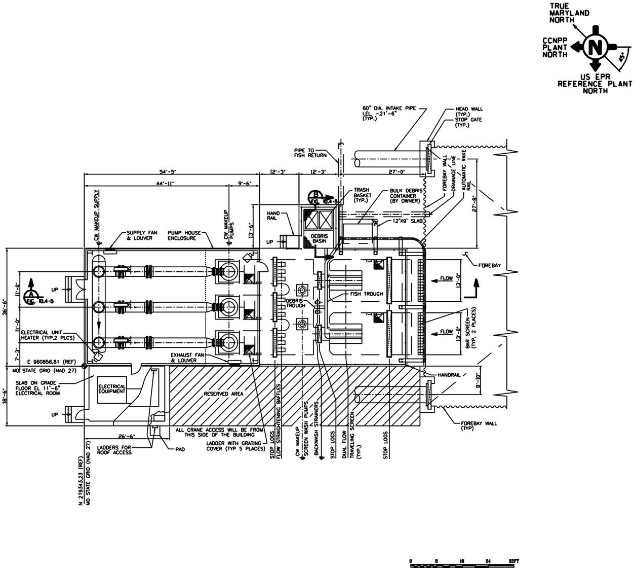
Figure 10.4-5—{Circulating Water System Makeup Pump Intake Structure (Section View)}
