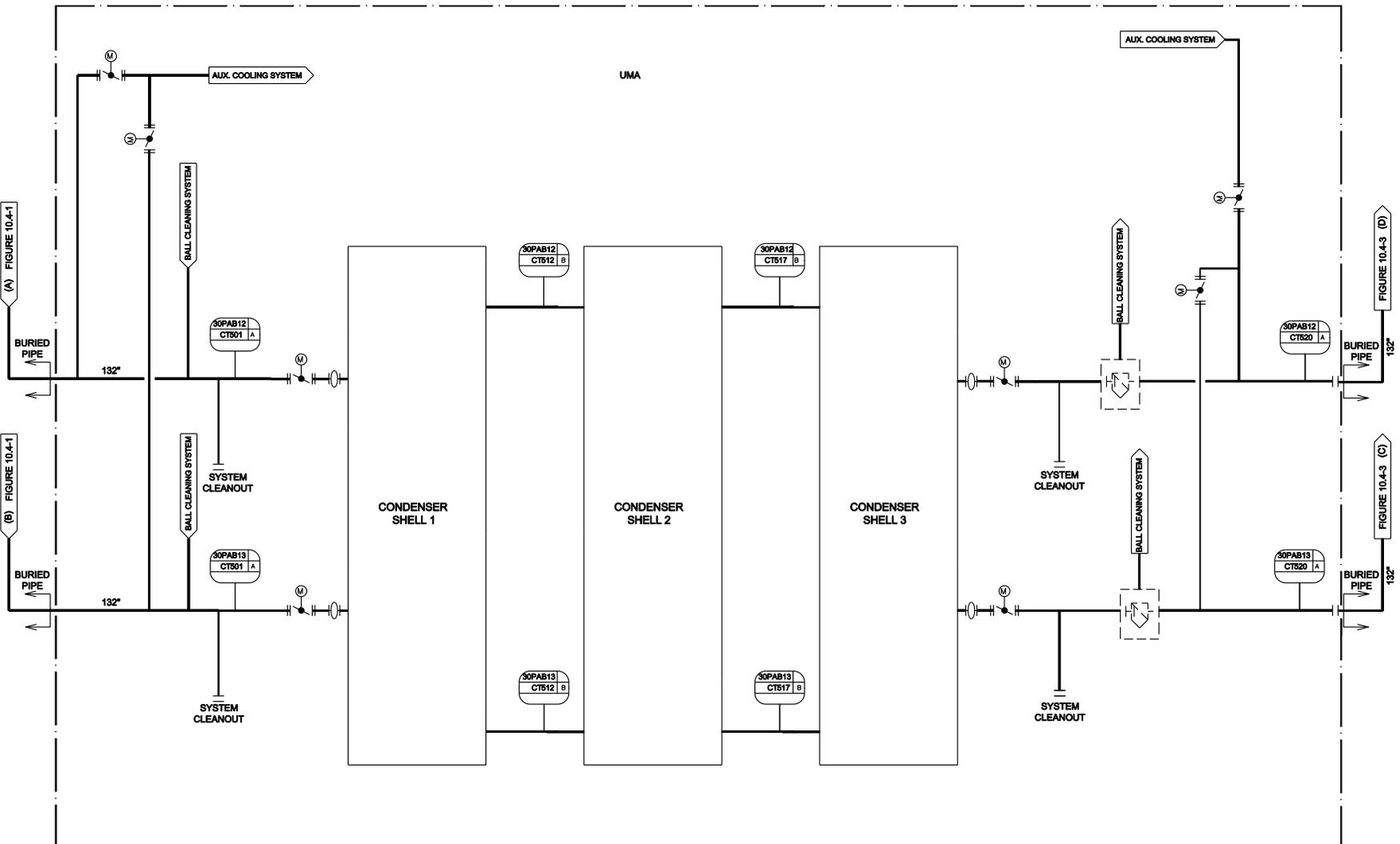
Figure 10.4-3—{Circulating Water System Makeup System P&ID}
