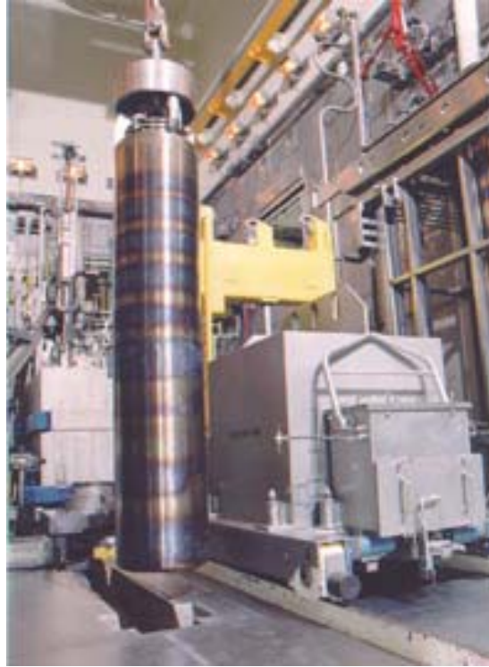
Figure 2.1 Canister containing vitrified (solidified in glass) high level waste at West Valley. (Photo from DEC.)
