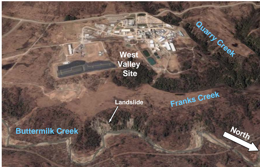
Figure 6.2 Three-dimensional representation of West Valley site. The site is perched on a terrace 200 feet above Buttermilk Creek, and cut through by Franks and Quarry Creeks, as well as Erdman Creek (not indicated but near "West Valley" label). Landslides also noted on Buttermilk Creek that are cutting towards the site. Vertical exaggeration is 2.5 times normal. (Image and topography from Google Earth.)
