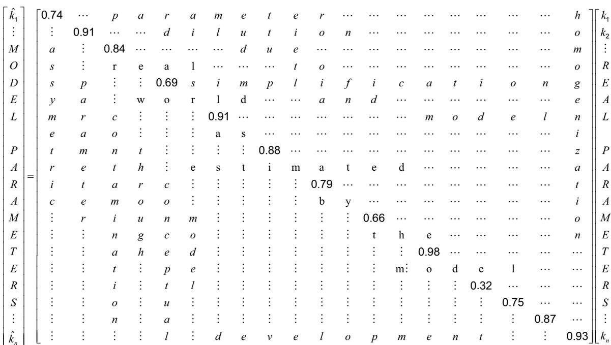
NOTES: Specifically, real-world parameters are averaged during the parameter estimation process required for model calibration. A better resolution matrix will have smaller off-diagonal elements (increased diagonal dominance) yielding model parameters that are closer approximations to the real parameters. Unfortunately, this can only occur where real-world heterogeneity is small and calibration data are ubiquitous and noise-free.
