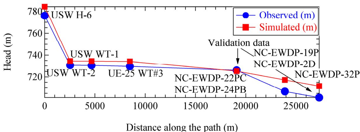
Figure 7-1b. Measured and Simulated Head Along Flowpath
