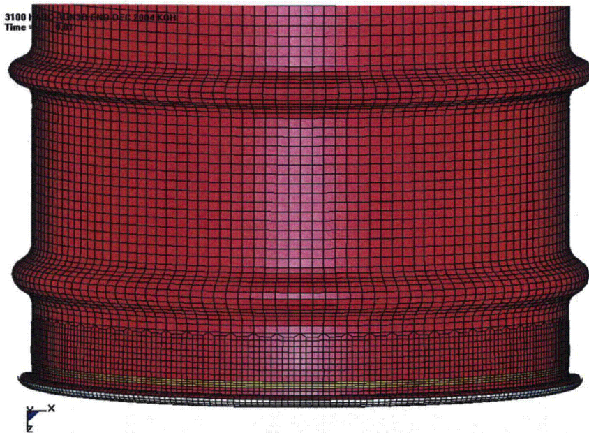
Figure 7.7.3.2 - HABC-Run3b, 30-Foot Impact Damage
