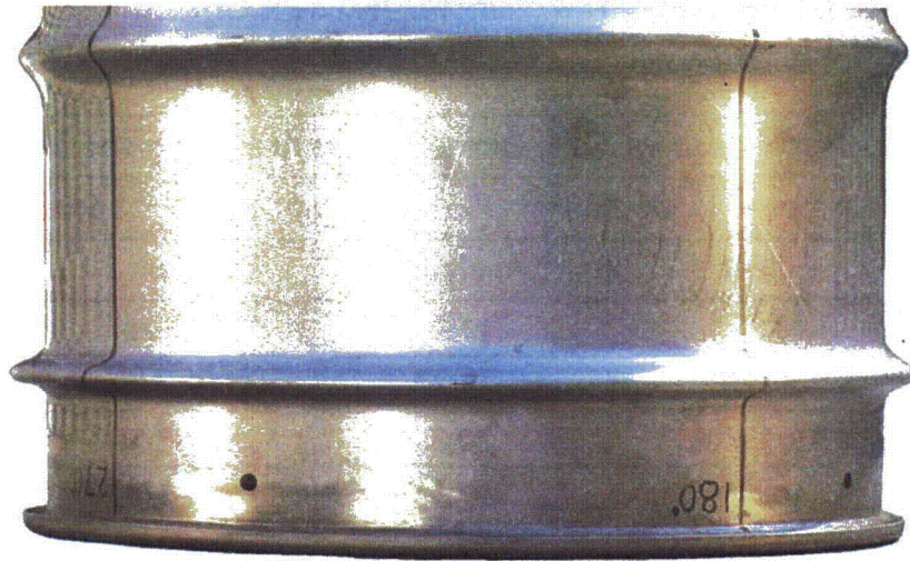
Figure 7.7.3.1 - TU4, 4-Foot + 30-Foot Impact Damage
