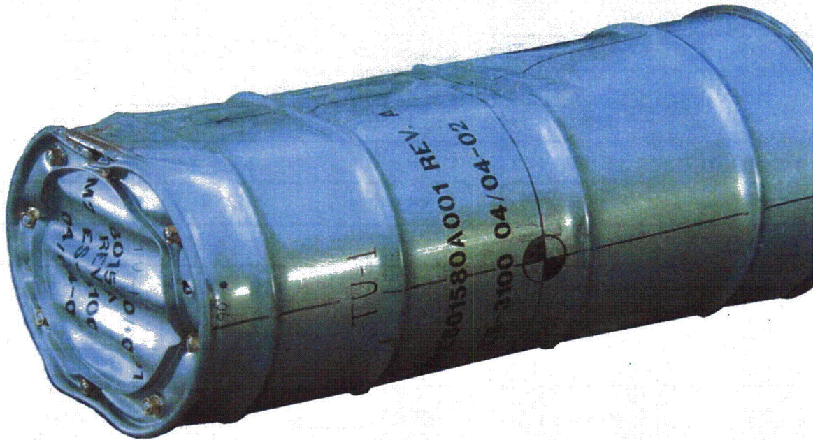
Figure 7.7.1.3 - TU1, View of Crush Damage with the Crush Side Up
