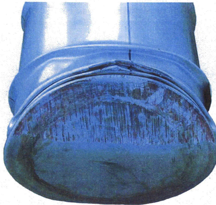
Figure 7.7.2.3 - TU3, Damage to the Bottom Head in the Crush Impact
