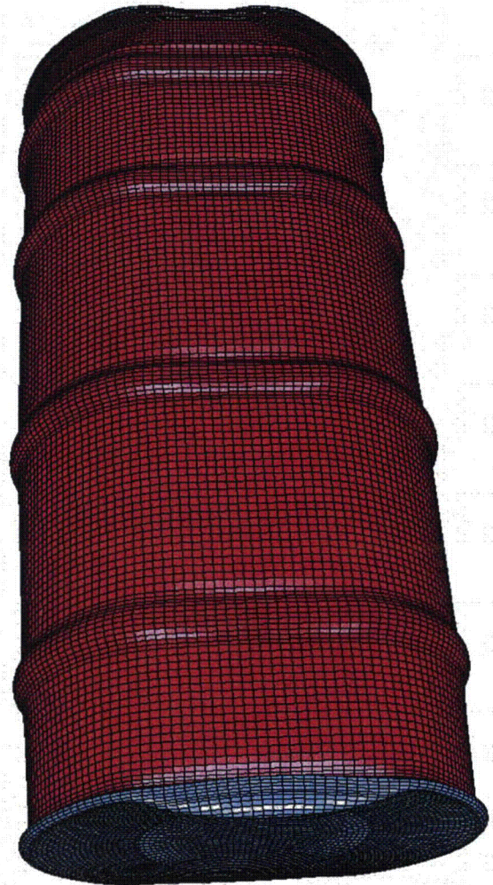
Figure 7.7.4.2 - HABC-run1hh, Cumulative Damage, Rigid Surface Side
