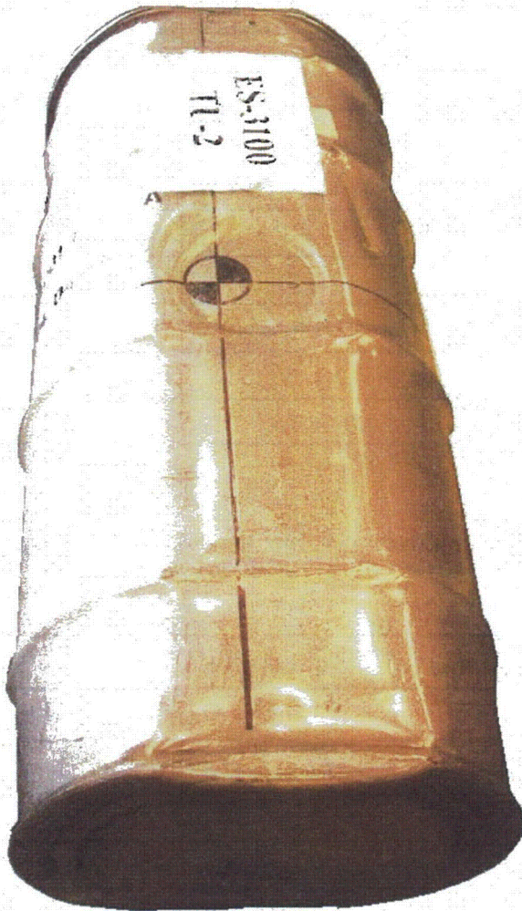
Figure 7.7.4.1 - TU2, Cumulative Damage After the Punch Impact, Rigid Surface Side
