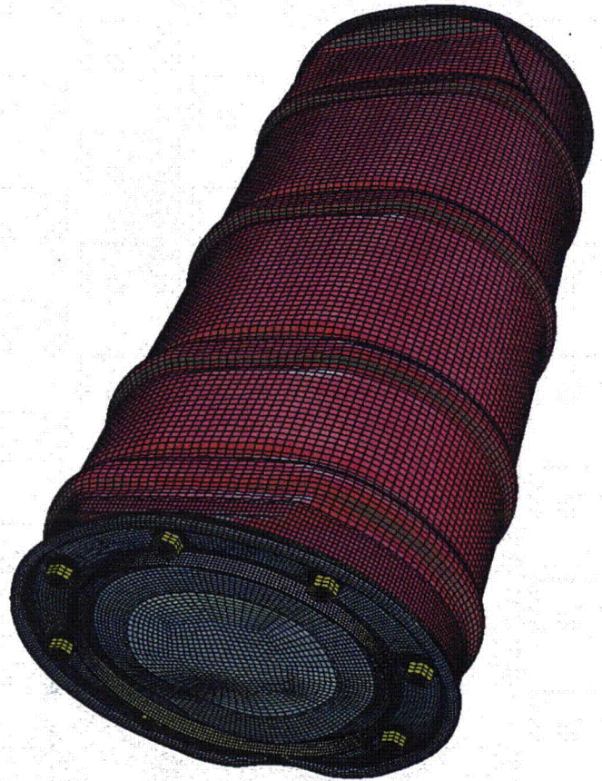
Figure 3.12.4.4 - Run1hh, Cumulative Damage After the Punch Impact, Crush Plate Side
