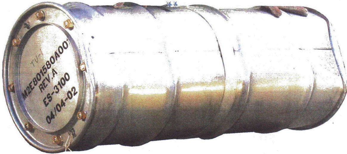
Figure 3.12.1.1 - TU1, Results of 30-Foot Impact
