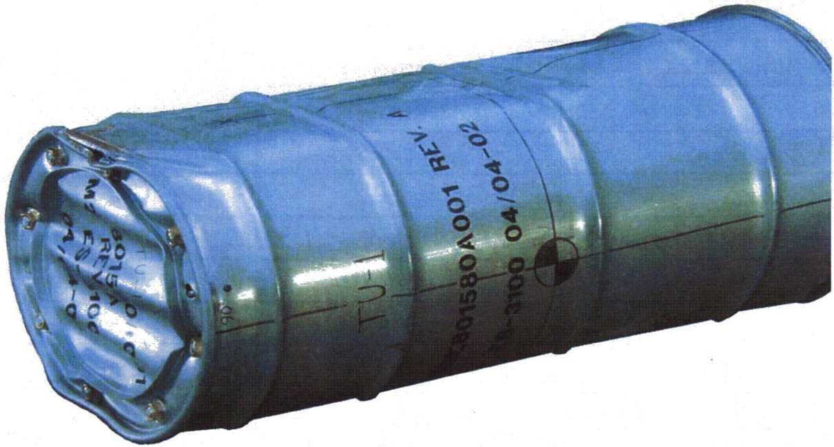
Figure 3.12.1.3 - TU1, View of Crush Damage with the Crush Side Up
