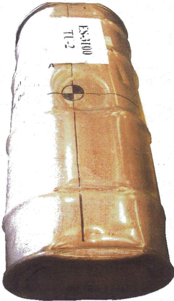
Figure 3.12.4.1 - TU2, Cumulative Damage After the Punch Impact, Rigid Surface Side
