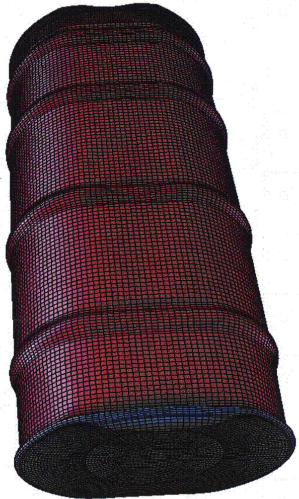
Figure 3.12.4.2 - Run1hh, Cumulative Damage After the Punch Impact, Rigid Surface Side
