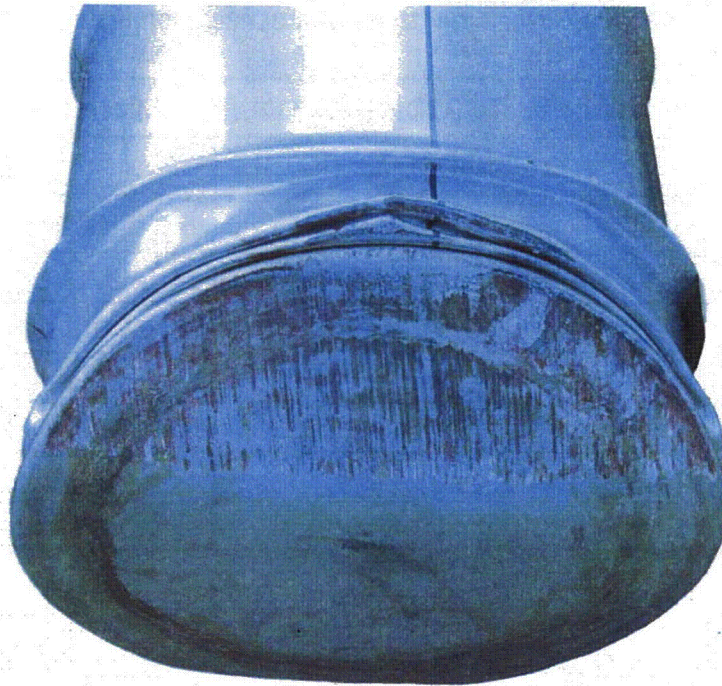
Figure 3.12.2.3 - TU3, Damage to the Bottom Head in the Crush Impact
