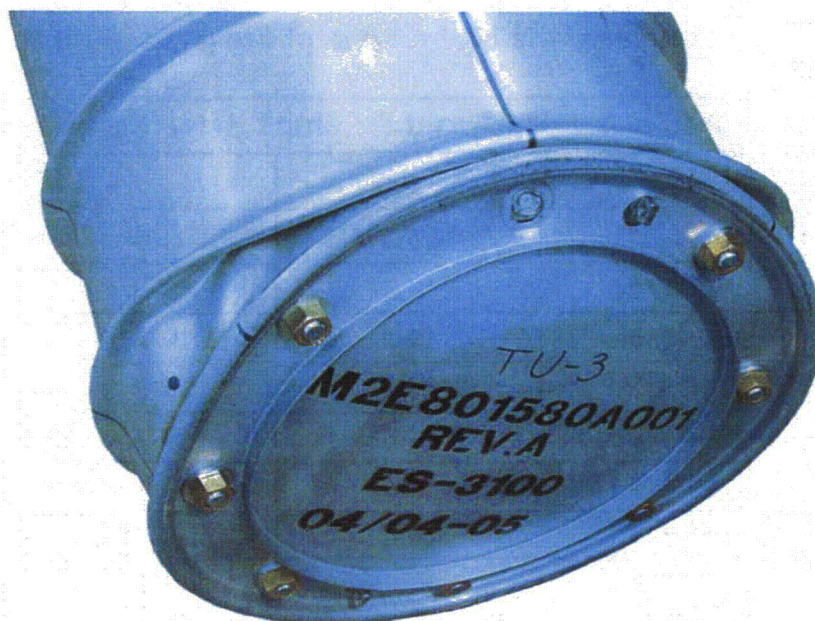
Figure 3.12.2.5 - TU3, Lid Damage from the Crush Impact
