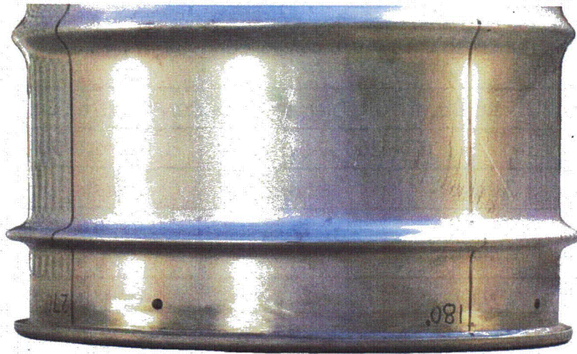
Figure 3.12.3.1 - TU4, 30-Foot Impact Damage
