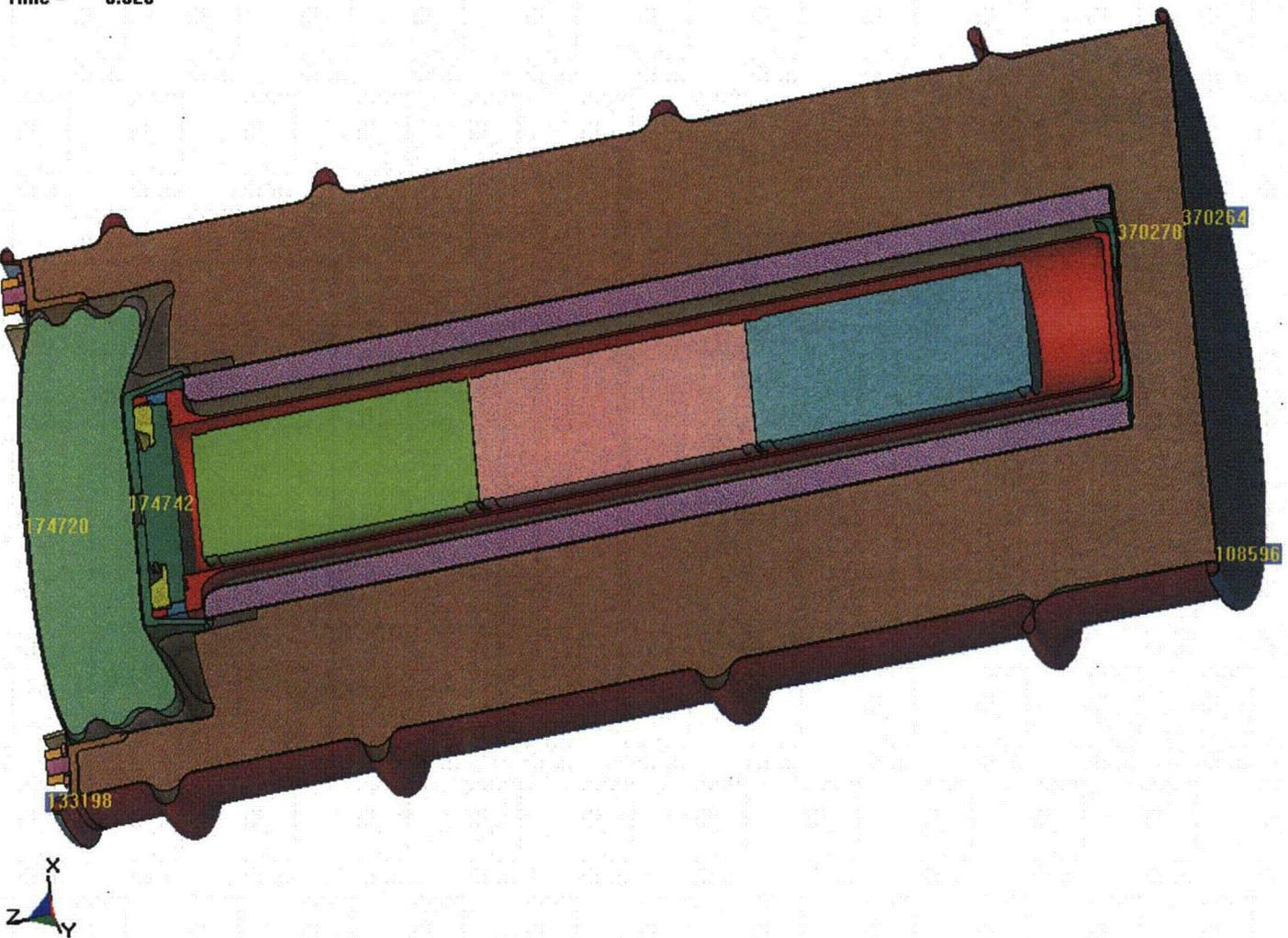
Figure 3.6.6 - Run3b, Nodes Chosen for Displacement Time Histories
