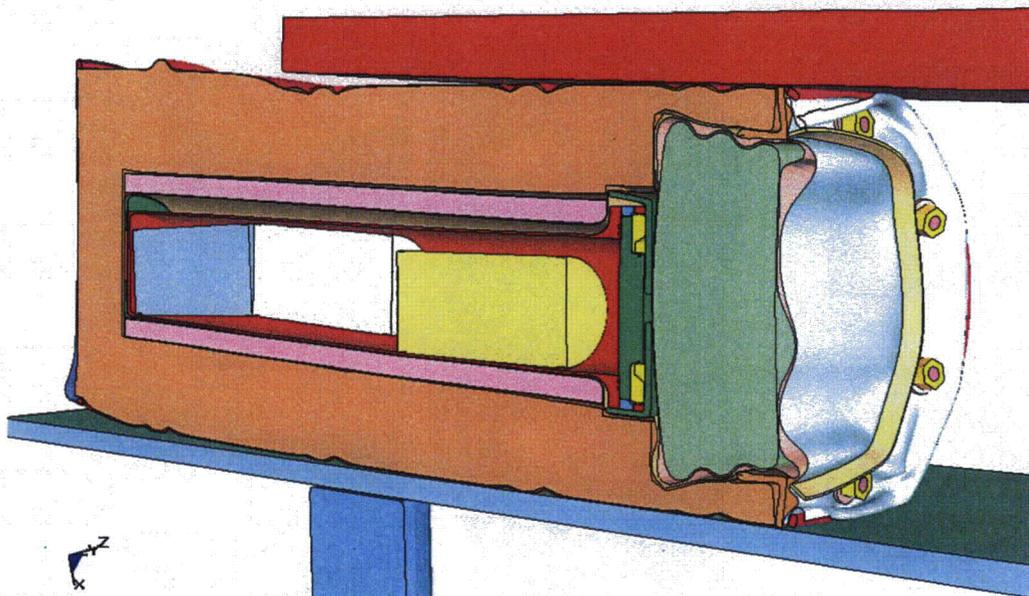
Figure 3.9.3 - Run4h, Crush Impact, Final Configuration
