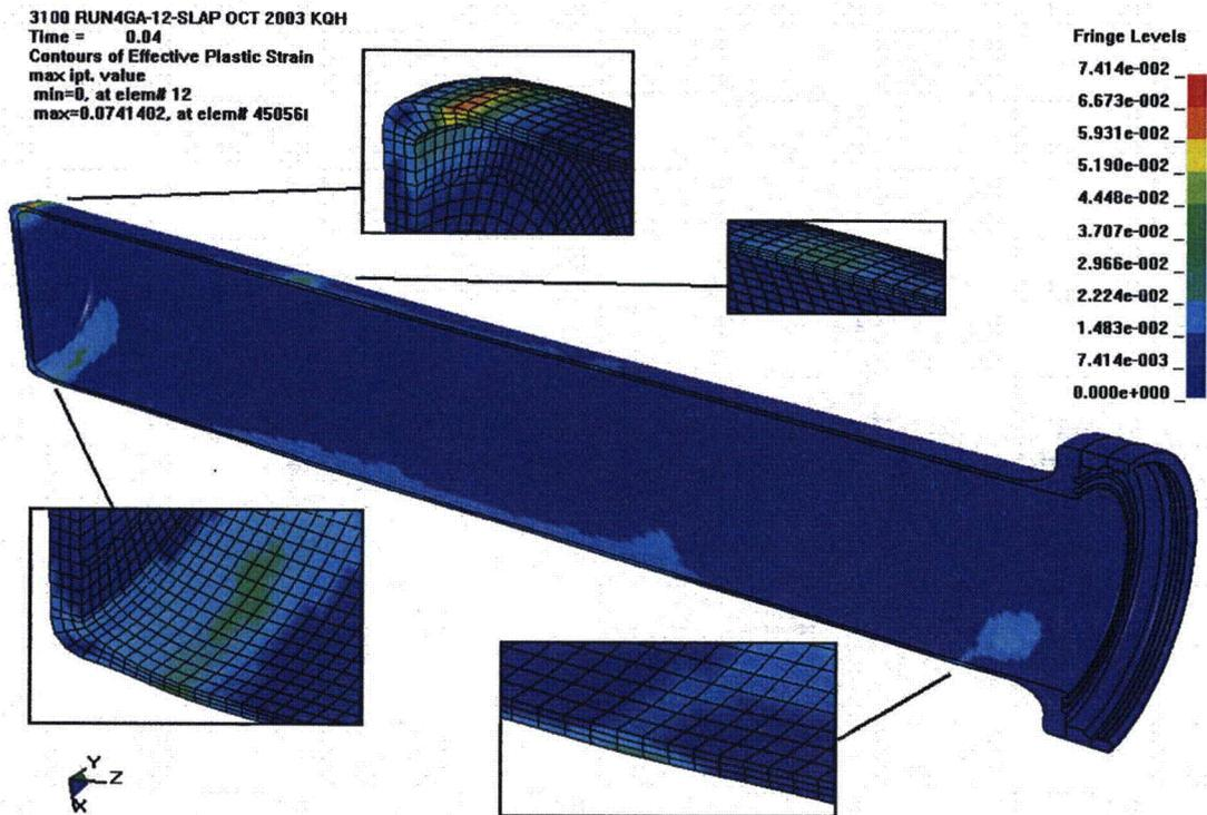
Figure 3.8.2 - Run4ga, Crush Impact, Effective Plastic Strain in the CV Body
