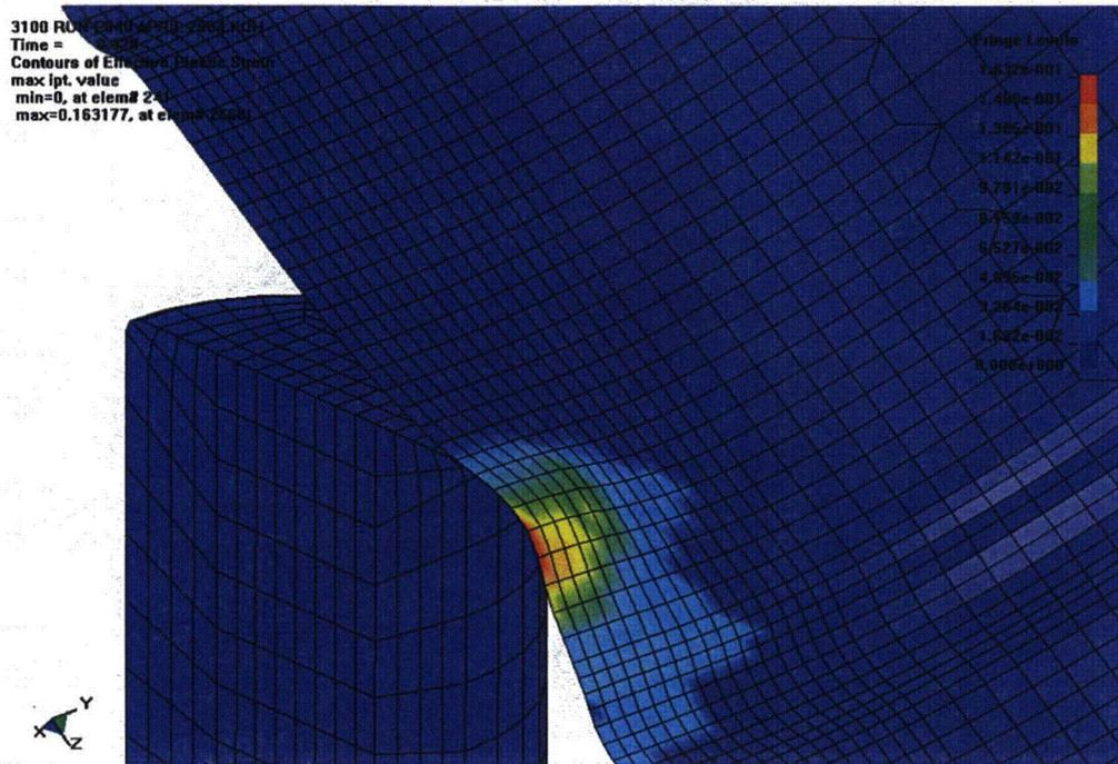
Figure 3.11.3 - Punch at 40°, Surface Strain in the Drum Liner
