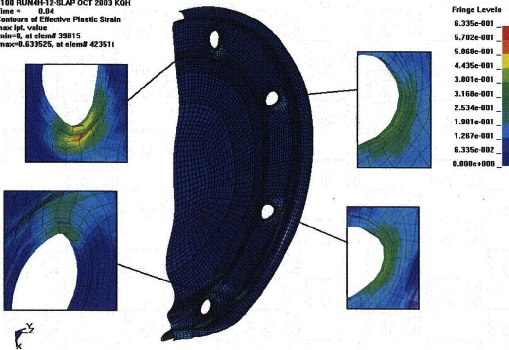
Figure 3.10.2 - Run4ha, Crush Impact, Effective Plastic Strain in the Lid
