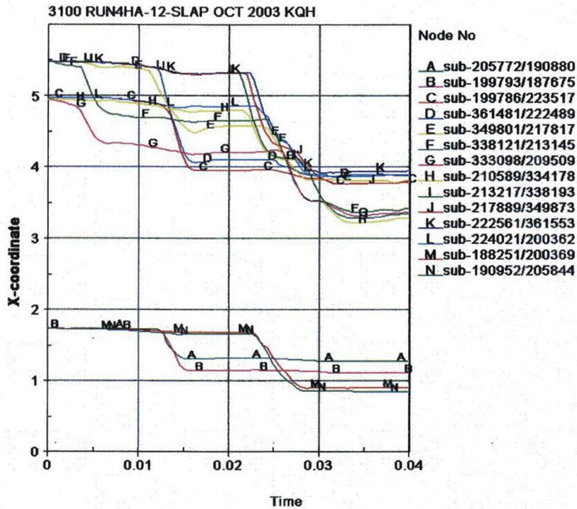
Figure 3.10.5 - Run4ha, Drum Kaolite Thickness in the Direction of the Impacts
