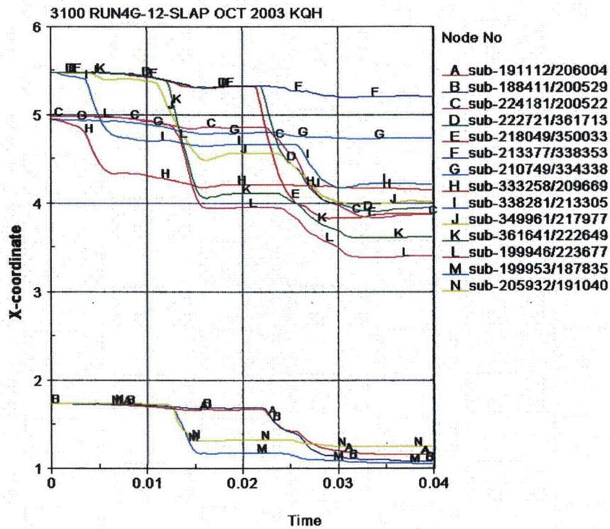
Figure 3.7.10 - Run4g, Kaolite Thickness Time Histories for the Impacts
