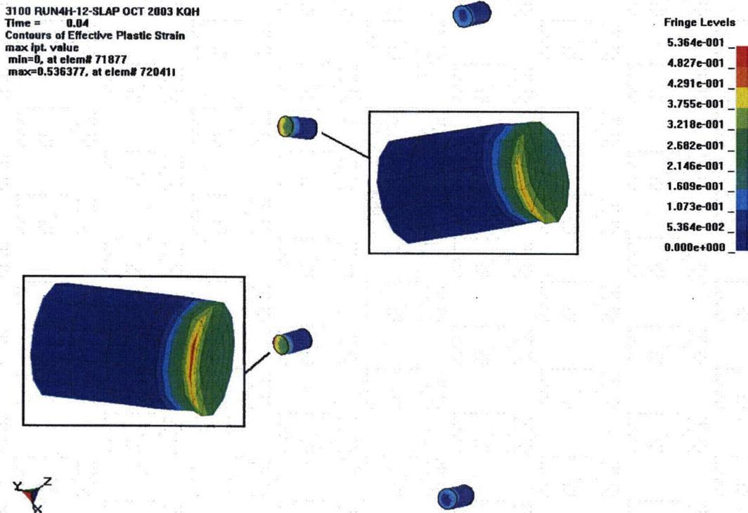
Figure 3.9.6 - Run4h, Crush Impact, Effective Plastic Strain in the Studs
