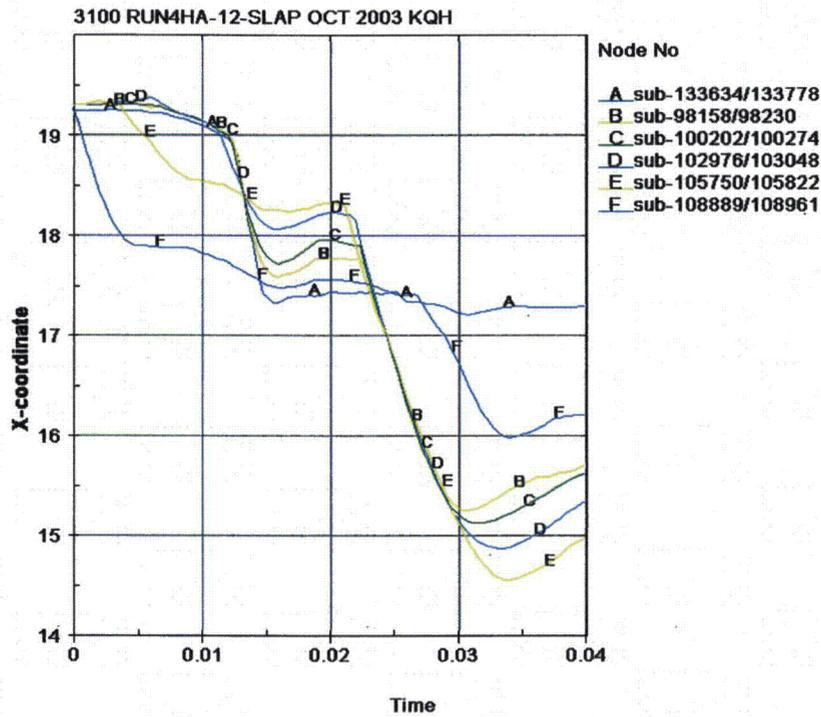
Figure 3.10.3 - Run4ha, Drum Diameter Time History in the Direction of the Impacts
