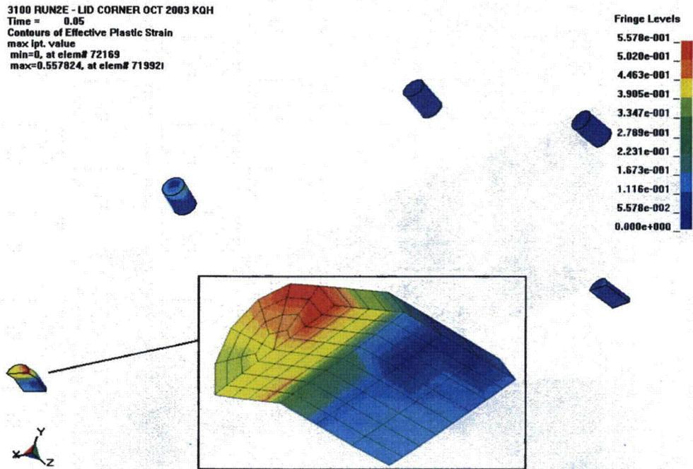
Figure 3.5.7 - Run2e, Crush Impact, Effective Plastic Strain in the Drum Studs
