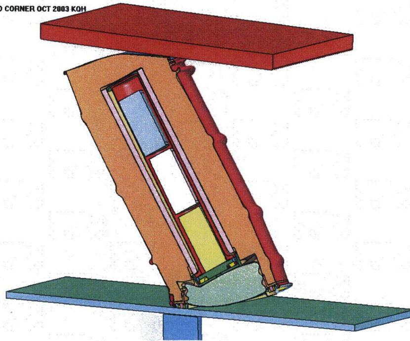
Figure 3.5.3 - Run2e, Crush Impact, Final Configuration
