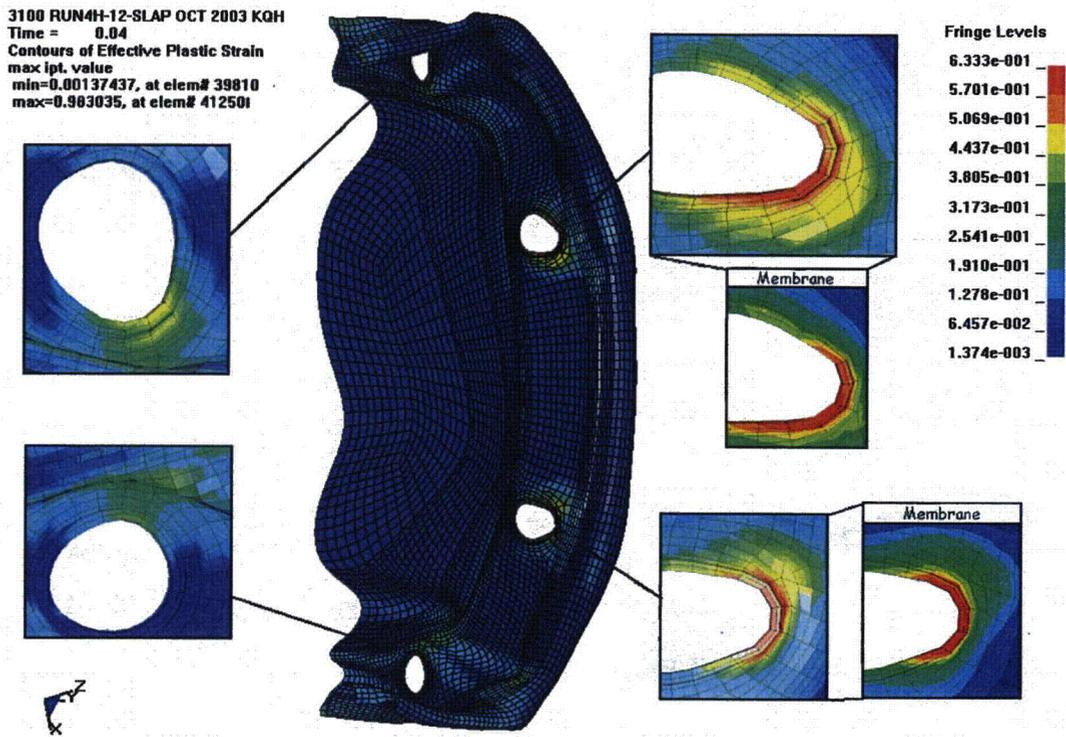
Figure 3.9.5 - Run4h, Crush Impact, Effective Plastic Strain in the Lid
