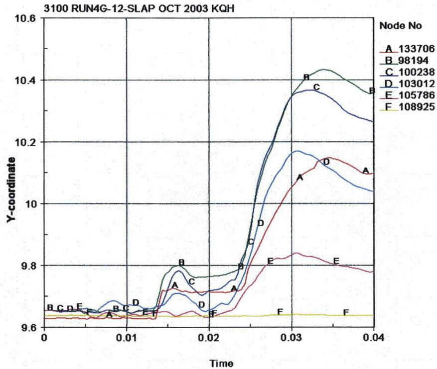
Figure 3.7.9 - Run4g, Drum Deformation Normal to the Impacts
