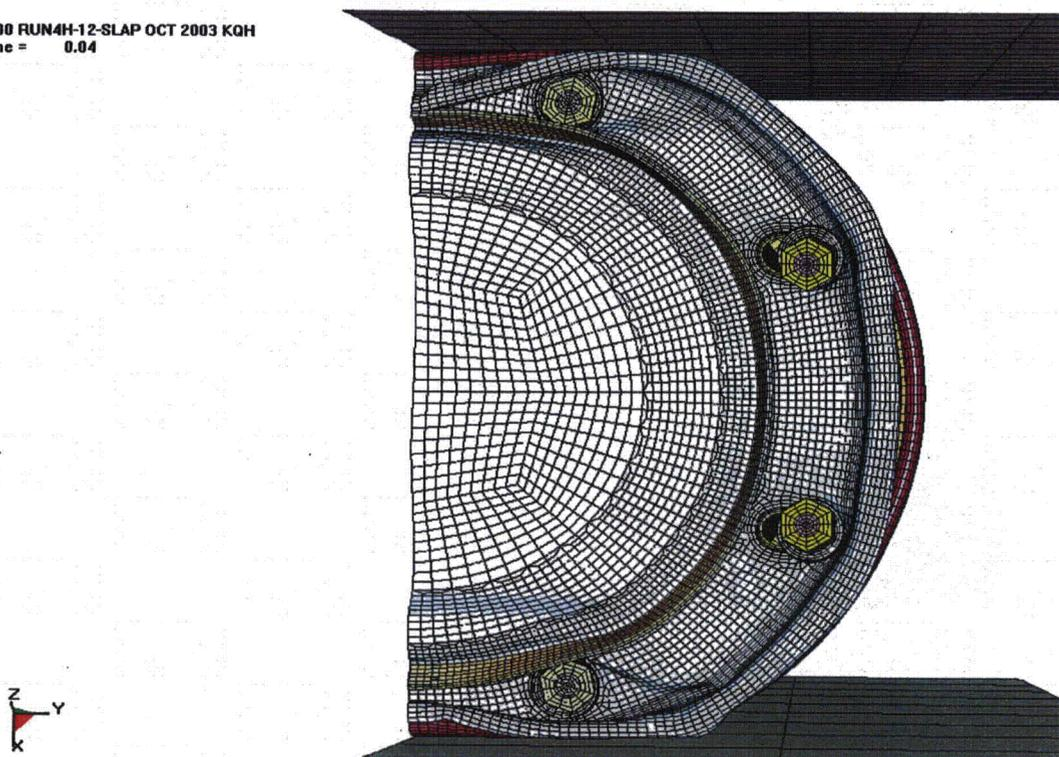
Figure 3.9.4 - Run4h, Crush Impact, Configuration of the Lid
