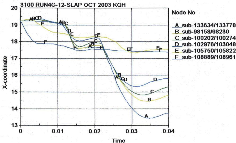
Figure 3.7.8 - Run4g, Drum Deformation in the Direction of the Impacts
