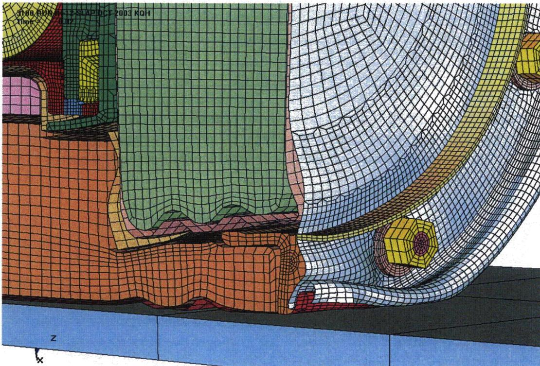
Figure 3.9.2 - Run4h, 30-Foot Impact, Configuration in the Lid
