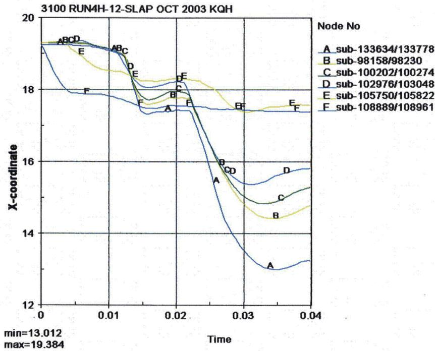
Figure 3.9.7 - Run4h, Drum Diameter in the Direction of the Impacts
