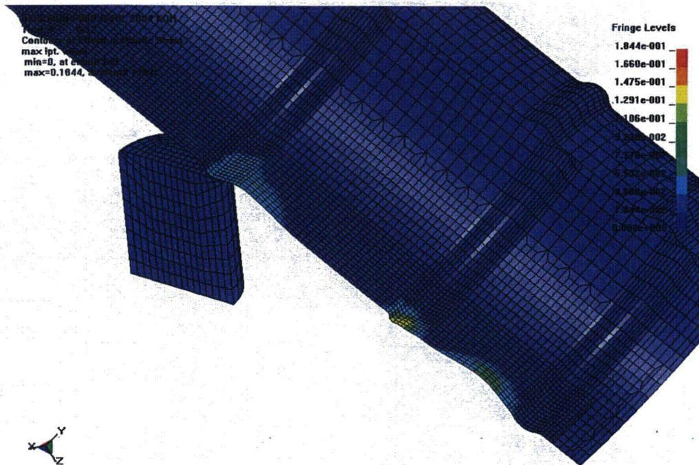
Figure 3.11.5 - Punch at 60°, Surface Strain in the Drum Liner
