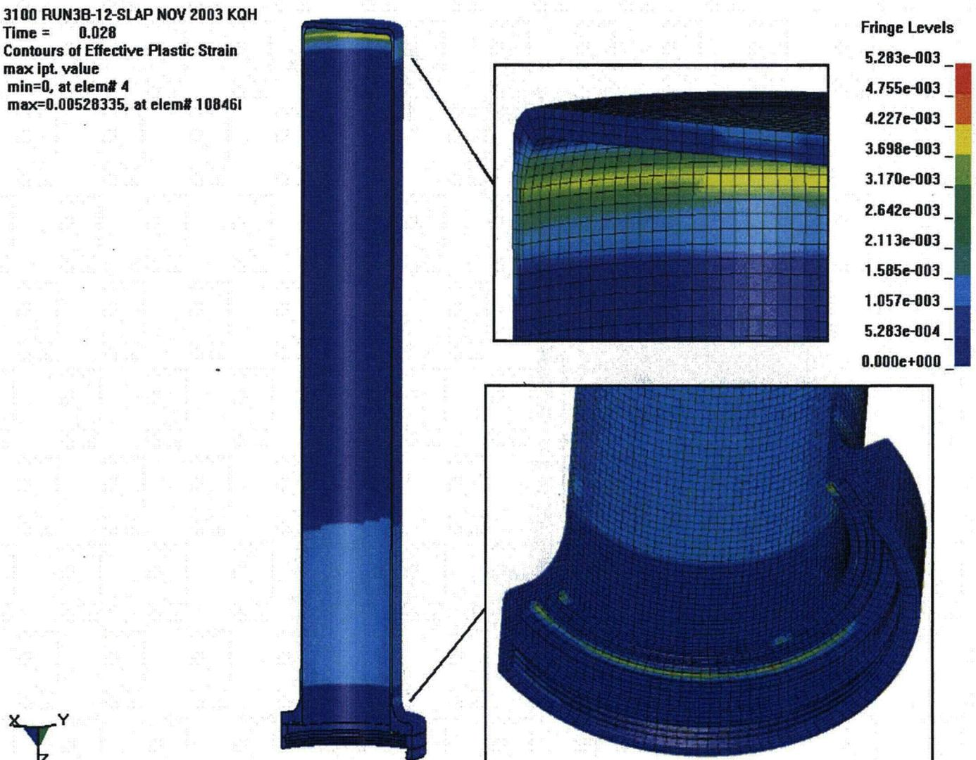
Figure 3.6.3 - Run3b, Crush Impact, Effective Plastic Strain in the CV Body
