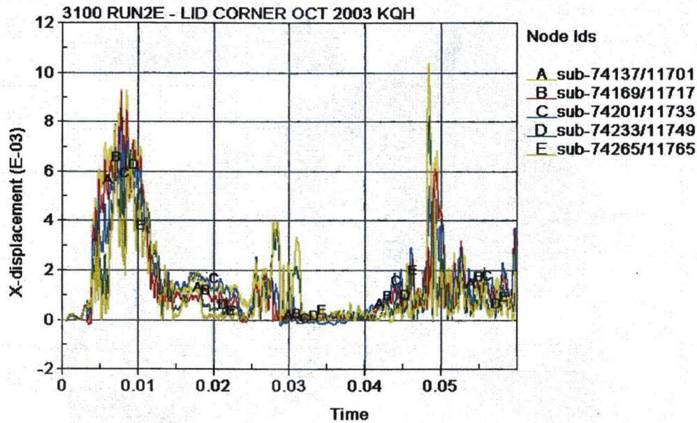
Figure 3.5.8 - Run2e, CV Lid/Body Separation Time History
