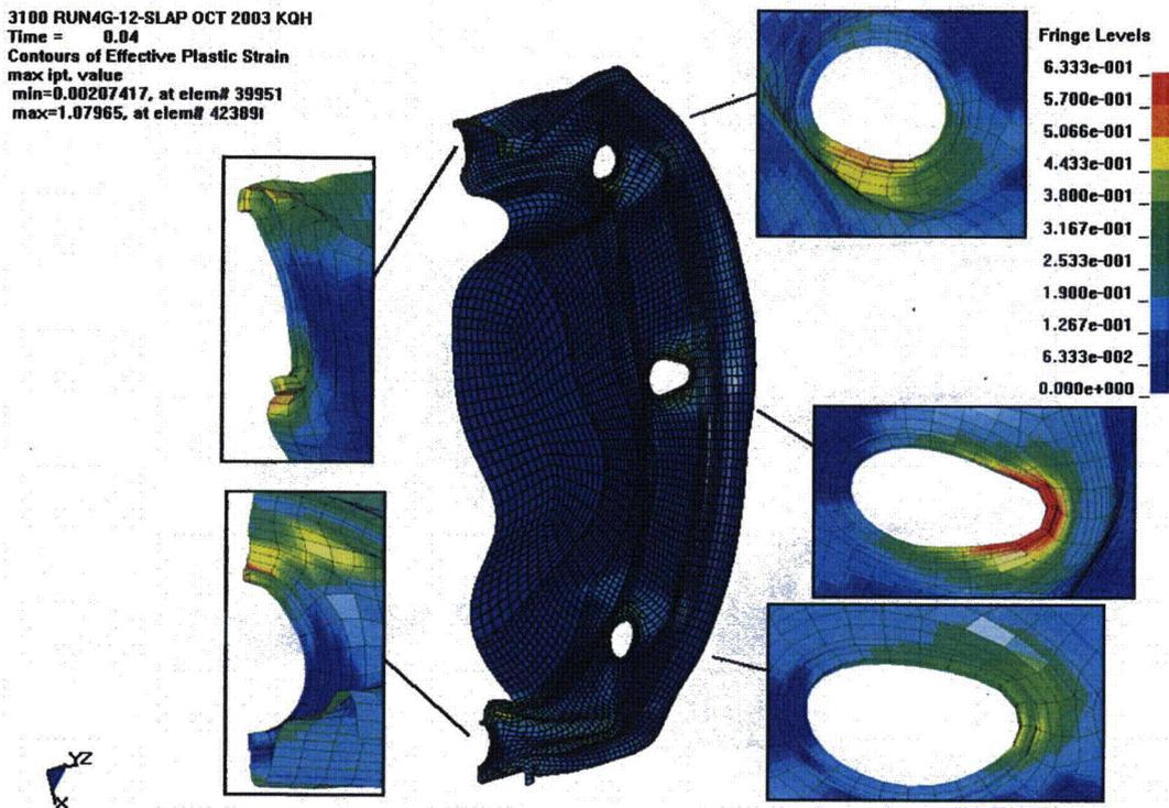
Figure 3.7.5 - Run4g, Crush Impact, Effective Plastic Strain in the Lid
