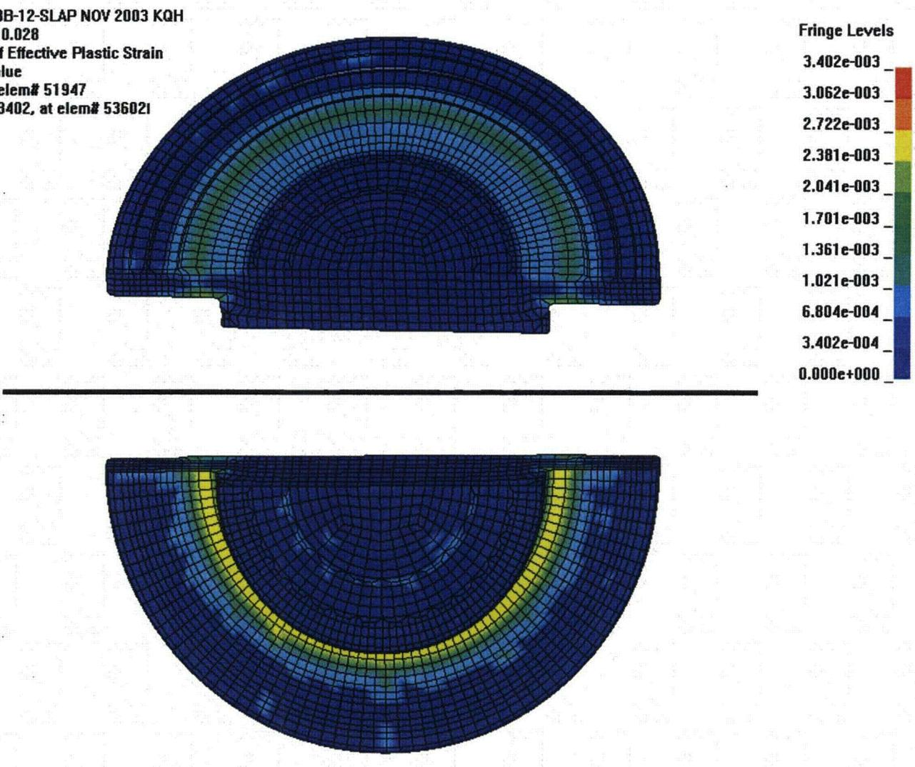
Figure 3.6.4 - Run3b, Crush Impact, Effective Plastic Strain in the CV Lid
