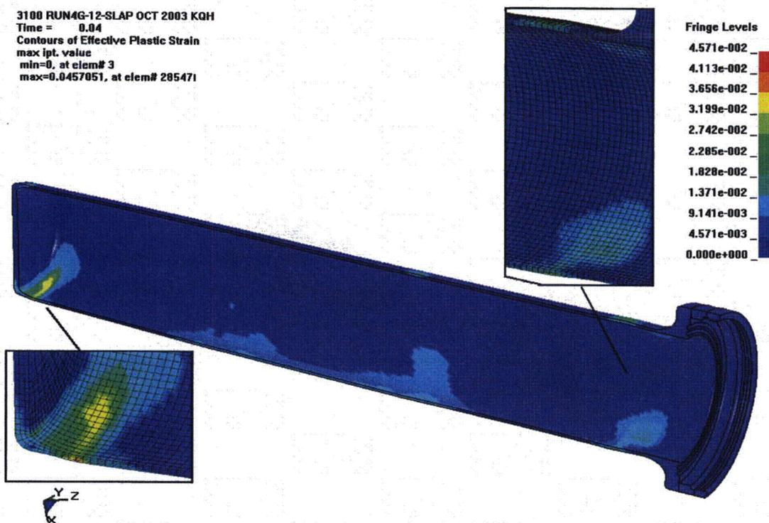
Figure 3.7.4 - Run4g, Crush Impact, Effective Plastic Strain in the CV Body
