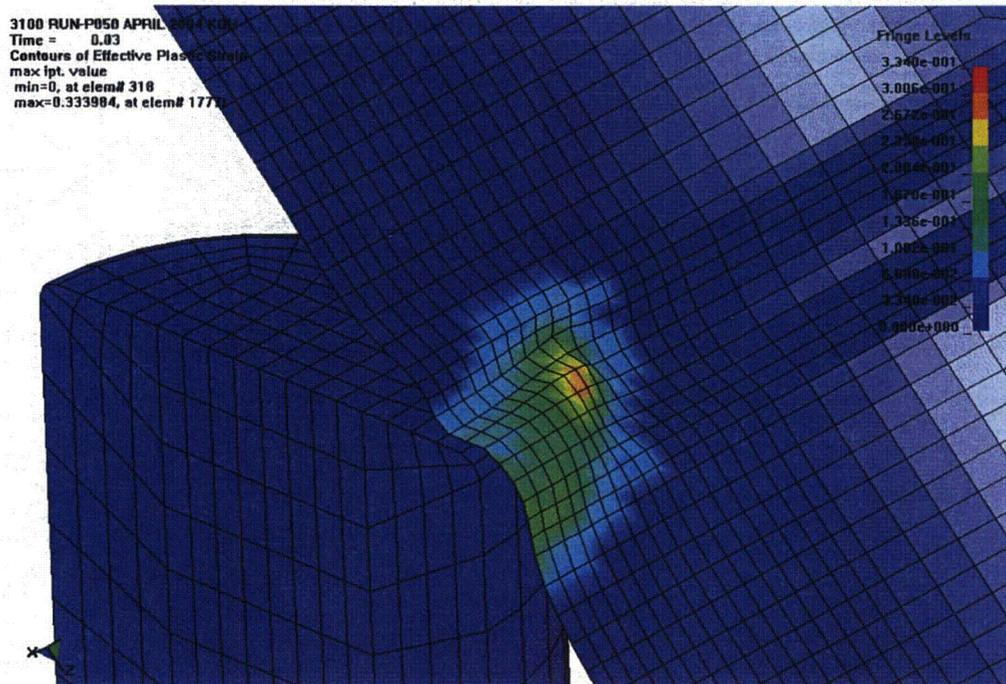
Figure 3.11.4 - Punch at 50°, Surface Strain in the Drum Liner
