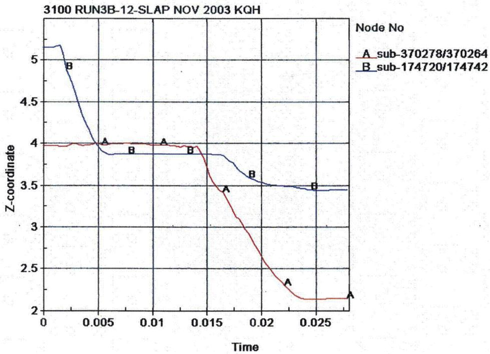
Figure 3.6.8 - Run3b, Kaolite Thickness Time History
