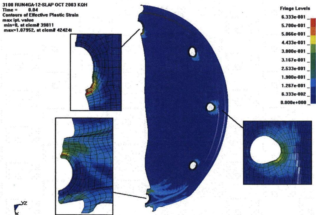
Figure 3.8.3 - Run4ga, Crush Impact, Effective Plastic Strain in the Lid
