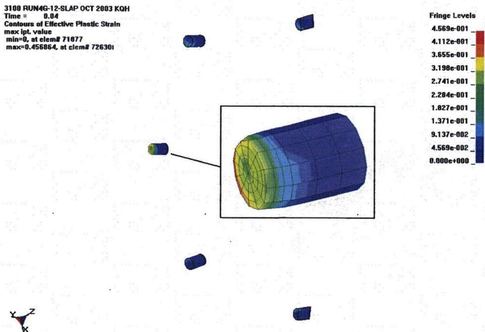
Figure 3.7.6 - Run4g, Crush Impact, Effective Plastic Strain in the Drum Studs
