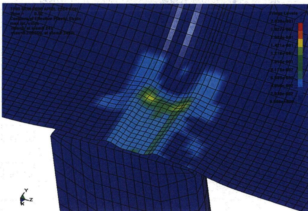
Figure 3.11.2 - Punch at 0°, Surface Strain in the Drum Liner
