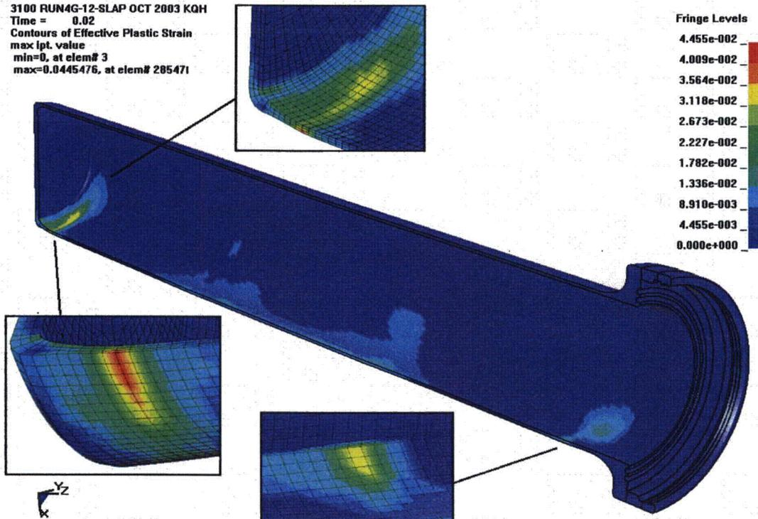
Figure 3.7.2 - Run4g, Slapdown Impact, Effective Plastic Strain in the CV Body
