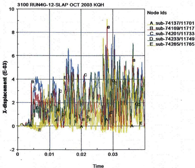
Figure 3.8.4 - Run4ga, Crush Impact, Lid Separation Time History
