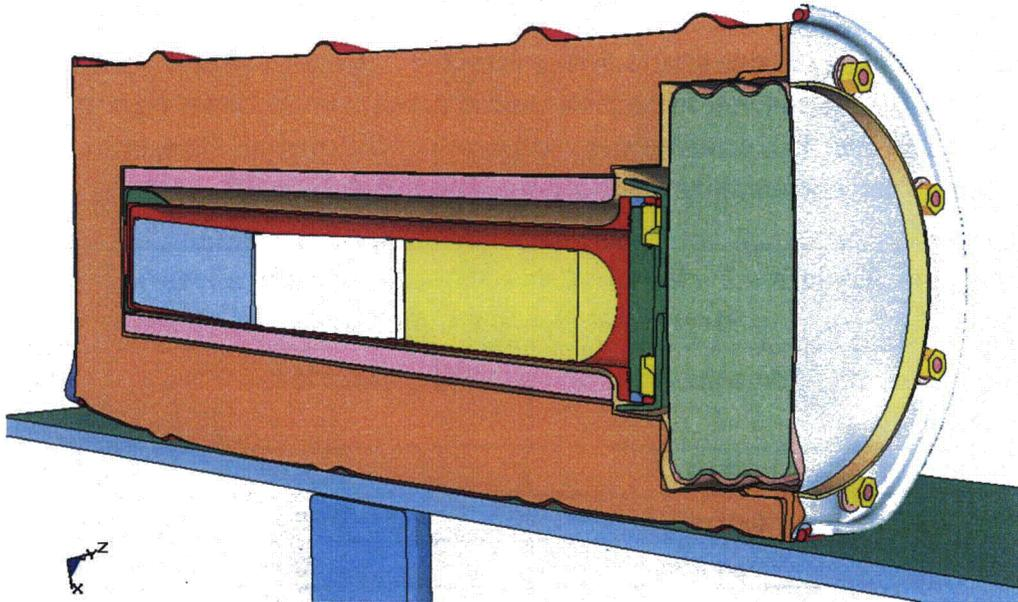
Figure 3.9.1 - Run4h, 30-Foot Impact, Final Configuration
