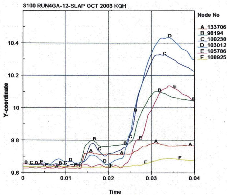
Figure 3.8.6 - Run4ga, Drum Deformation Time History in the Y-Direction
