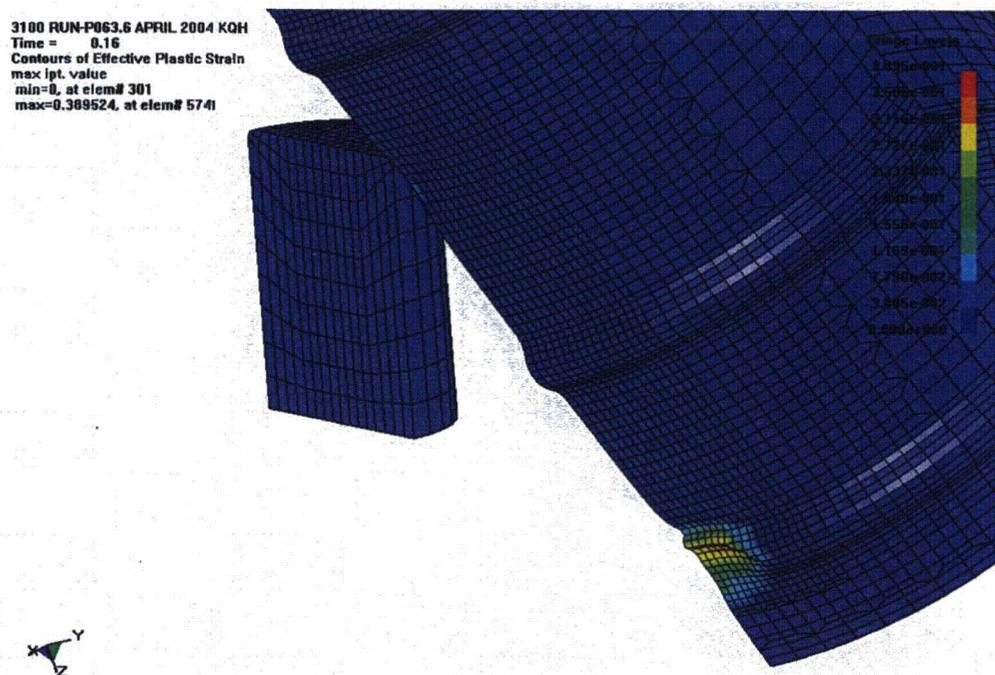
Figure 3.11.6 - Punch at 63.6°, Surface Strain in the Drum Liner
