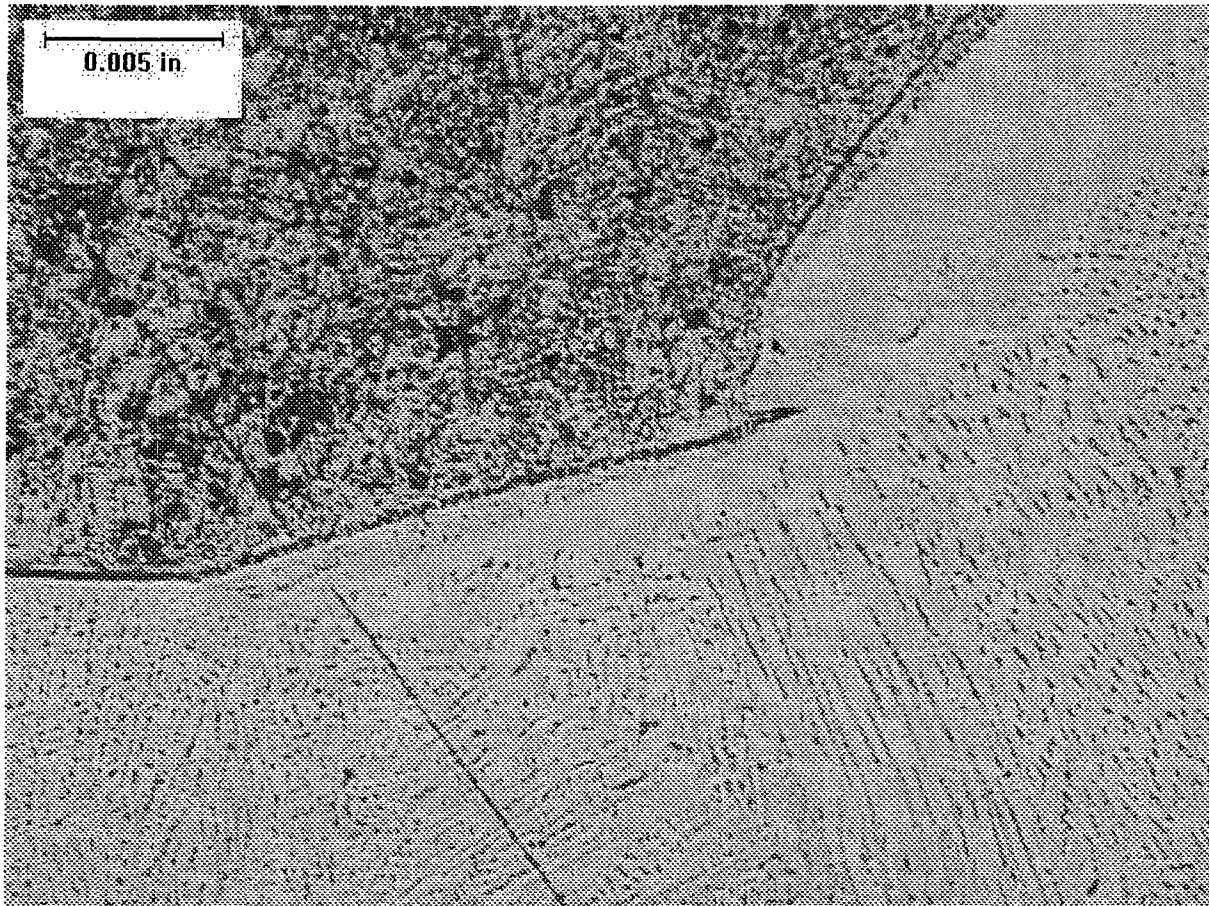
Figure 25 Metallography Results Illustrating the Typical Microstructures of the Carbon Steel and Weld Metal in Sample A3B
