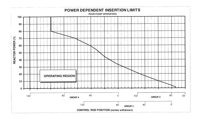
Figure 2.2-1 Regulating Rod Group Position Limits
