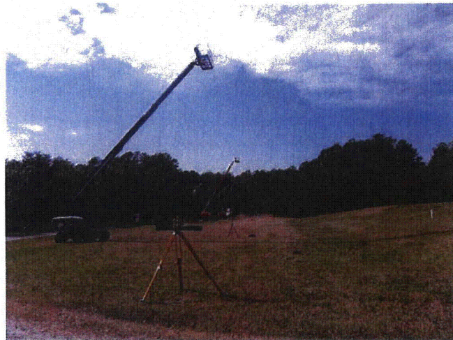
Figure 7 Microphone measurement positions at the GTRI outdoor test site.
