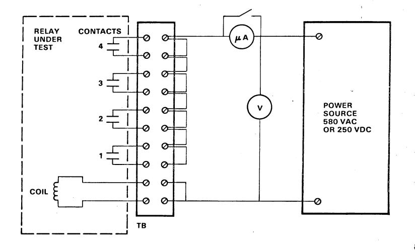
Figure 9.2. Coil-to-Contact Leakage Current
