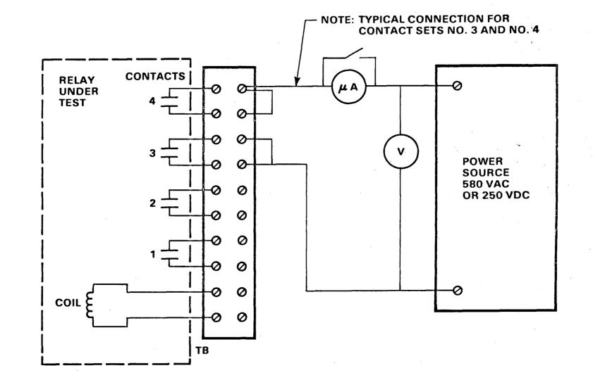
Figure 9.4. Leakage Current Between Contacts
