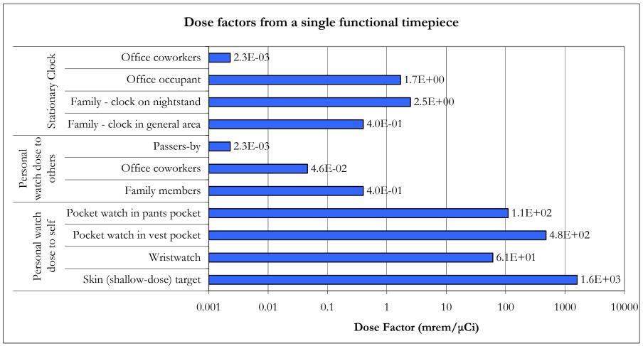
Figure 3) Dose factors from a single functional timepiece
