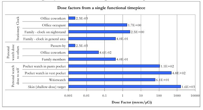
Figure 1) Dose factors from a single functional timepiece
