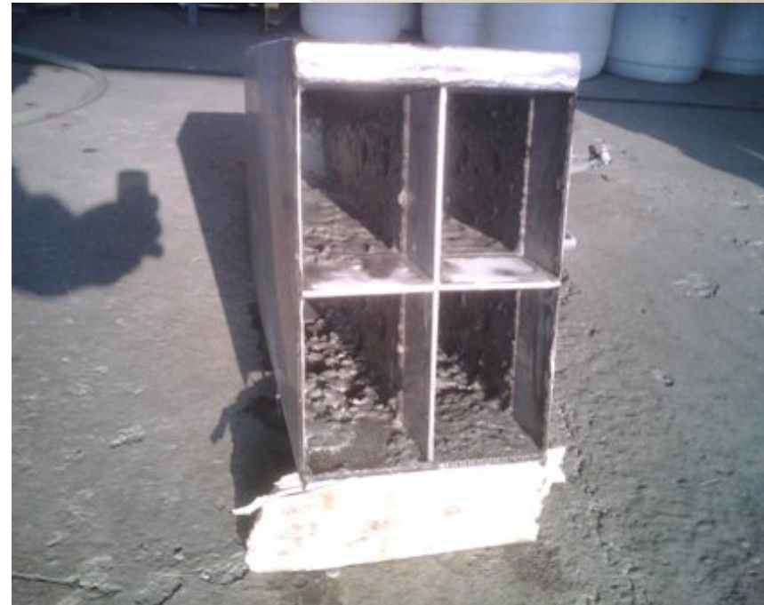
Post Test Debris Loaded Screen
