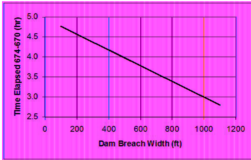
Figure 4. Chickamauga Dam breach width versus elapsed time of the reservoir recession level from 674 ft-msl to 670 ft-msl. This plot was re-constructed based on the licensee's simulations of recession rates using the SOCH model with an initial reservation level of 675 ft-msl (Ref. 3).
