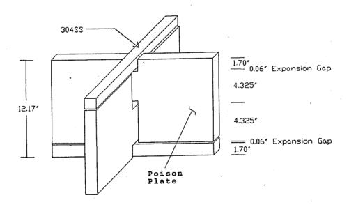
A 0.94 in. total width gap exists between the plates in the slots.
