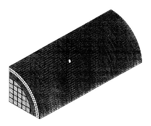
FIGURE 3-5 FINITE ELEMENT PLOT OF THE TN-68 IMPACT LIMITERS MODEL
