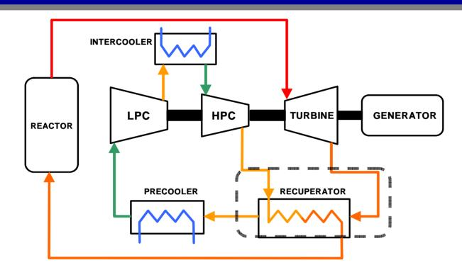
Recover heat from the turbine exhaust stream and transfer it to the reactor helium inlet stream
