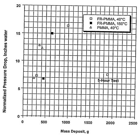
Figure 5. Gaskill small scale tests using PMMA fuel.—Data taken from Figure 4.
