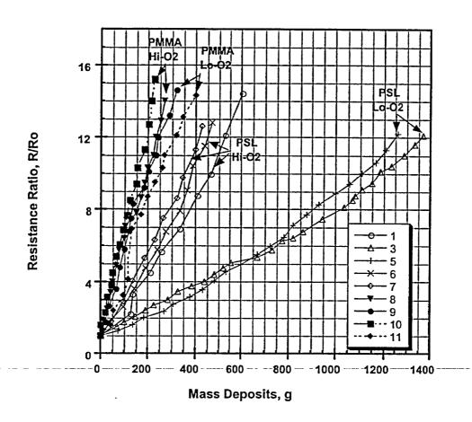
Figure 1 Summary of Fenton et al data on smoke loading using a small scale smoke generator (Battel generator) and full-scale (1,000 cfm) HEPA filter.
