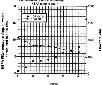
Figure 10. Gaskill large scale test No. 1 with a scrubber (not shown), Note the pressure drop (normalized to 1,000 cfm) across the HEPA filter increases continuously with increasing time. This tests shows the scrubber does not protect the HEPA filter.
