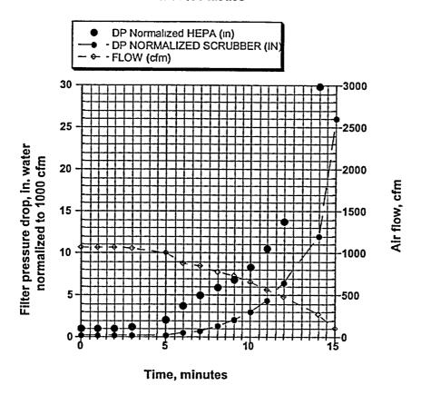
Figure 11. Gaskill large-scale tests with a scrubber shows the HEPA plugs rapidly..
