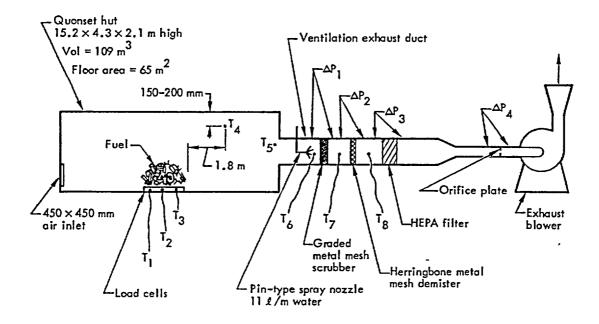
Figure 9. Gaskill large-scale tests with full-scale (1,000 cfm) HEPA filter. Smoke generated inside chamber.
