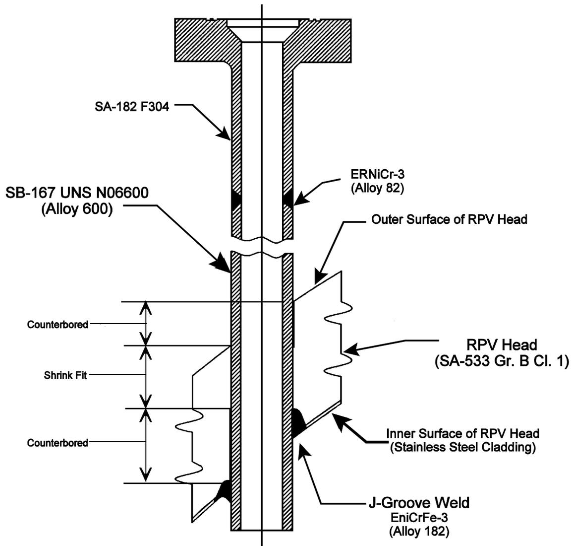
Figure 1. Schematic of Typical CRDM Nozzle Penetration
