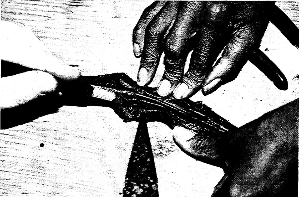
**Figure 3.17** Dissected splice from a Group 3.4 specimen after LOCA testing
