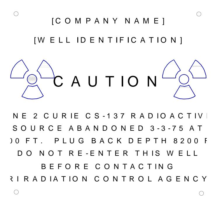
The size of the plaque should be convenient for use on active or inactive wells [e.g. a 7-inch square]. Letter size of the word "CAUTION" should be approximately twice the size of the rest of the information. [e.g. 1/2 inch and 1/4 inch letter size, respectively.]
