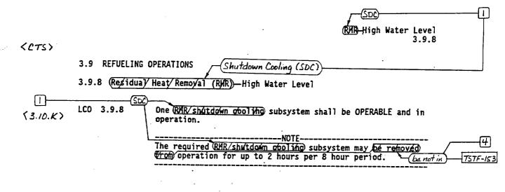
(App/ 3.10.K) APPLICABILITY: MODE 5 with irradiated fuel in the reactor pressure vessel
