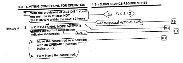
In OPERATIONAL MODE 5, this Specification is applicable for withdrawn control rode and is not applicable to control rode and is not applicable to control rode removed per Specification 3.10 y or 3.18.J
