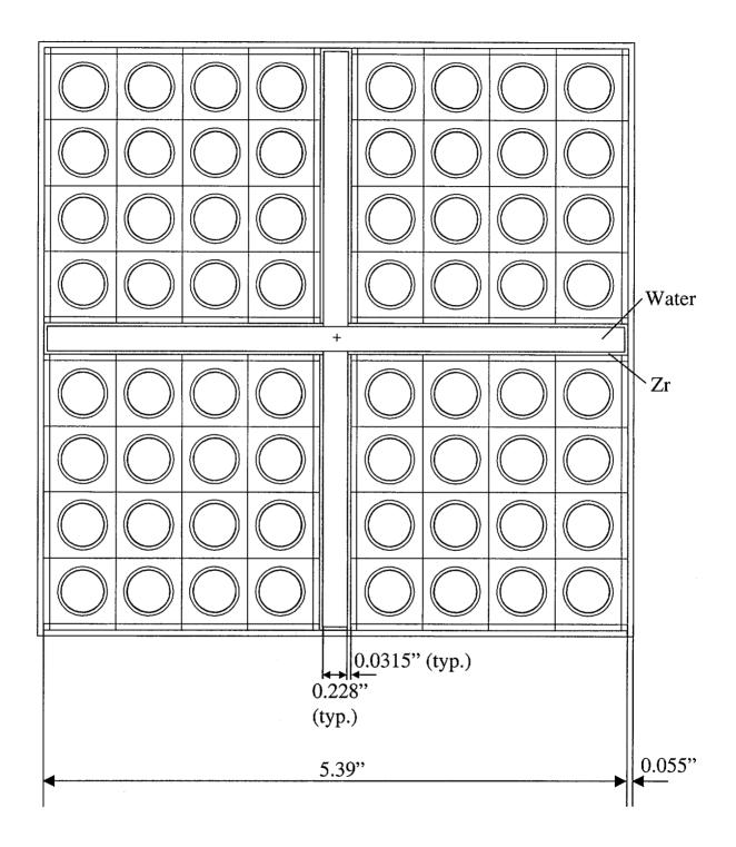
MCNP Model of QUAD+ Assembly with Dimensions
