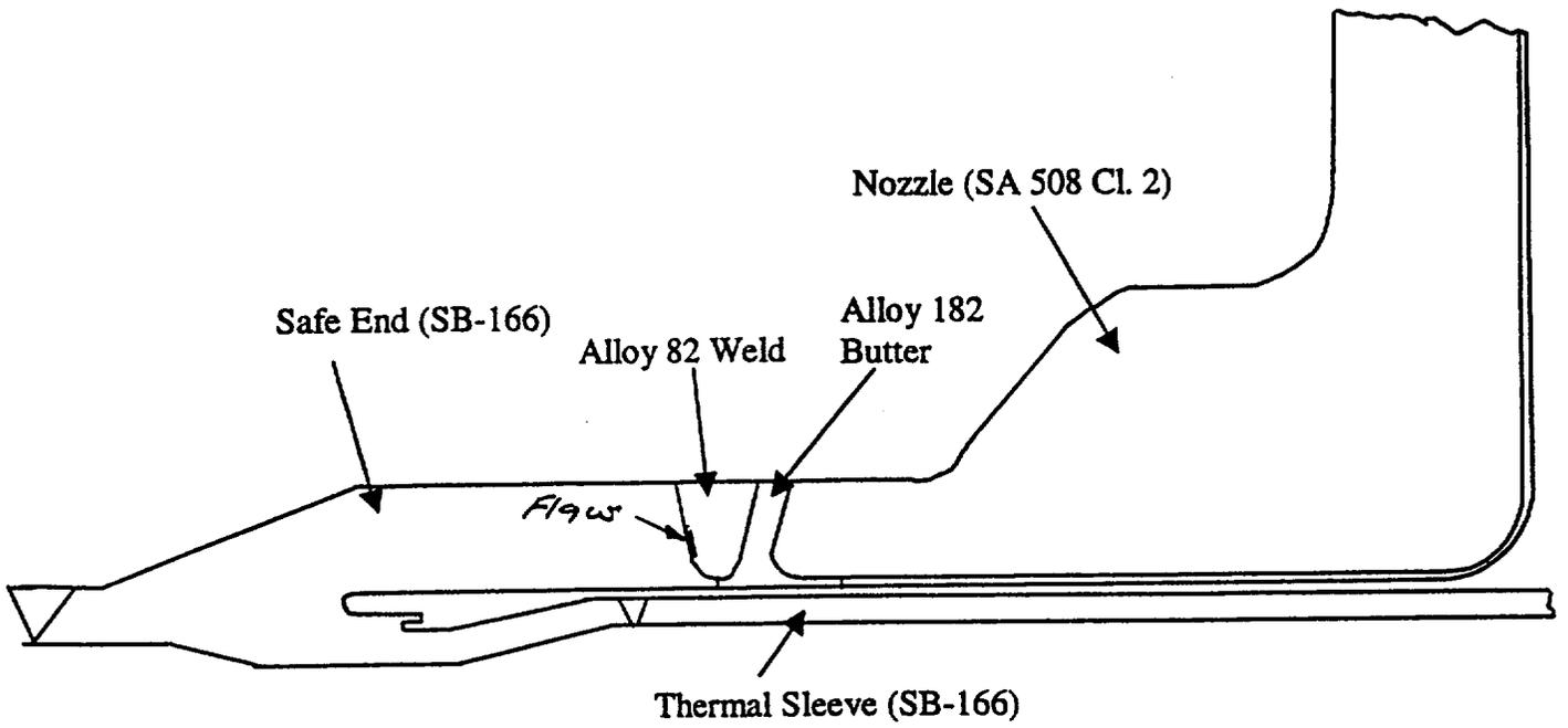
Figure 1. Flaw in Recirculation Inlet Nozzle N2F
