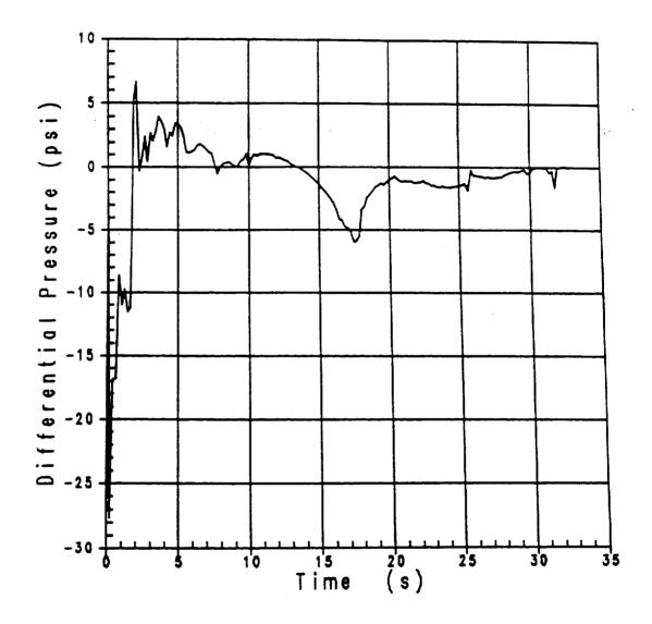
Figure 3.1-16 Core Pressure Drop Uprating Analysis - RHR Crosstie Closed,  $F_q = 2.335$
