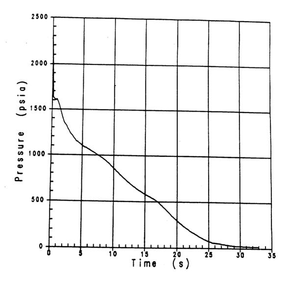
Figure 3.1-14 Reactor Coolant System Pressure Uprating Analysis - RHR Crosstie Closed,  $F_{\alpha}$  = 2.335
