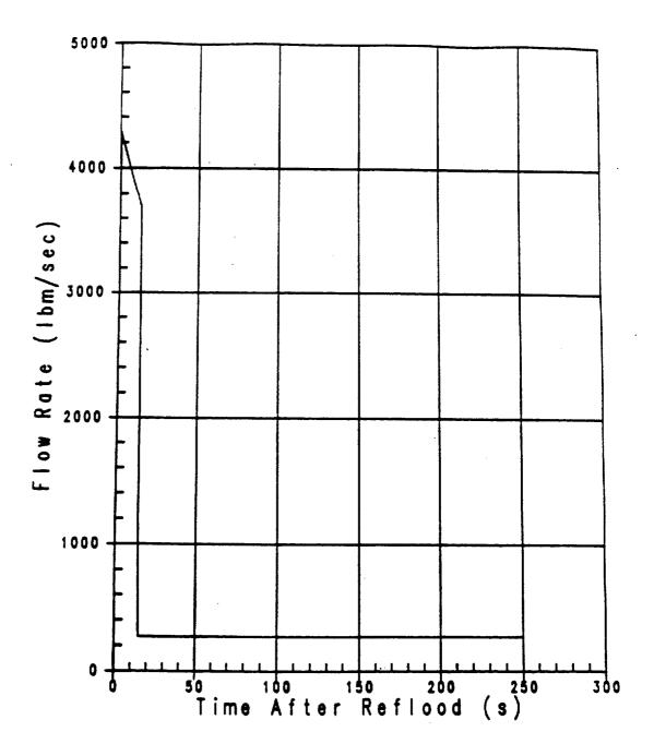
Figure 3.1-8 Accumulator and SI Flow During Reflood Uprating Analysis–RHR Crosstie Closed
