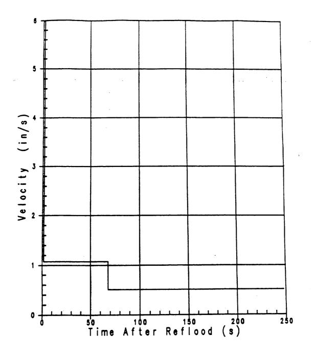
Figure 3.1-7 Core Inlet Flow During Reflood Uprating Analysis–RHR Crosstie Closed
