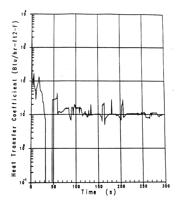
Figure 3.1-11 Rod H.T.C. at Peak Temperature Elevation Uprating Analysis–RHR Crosstie Closed
