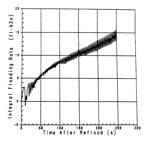
Figure 3.1-22 Integral of Core Inlet Flow Uprating Analysis - RHR Crosstie Closed,  $F_q = 2.335$
