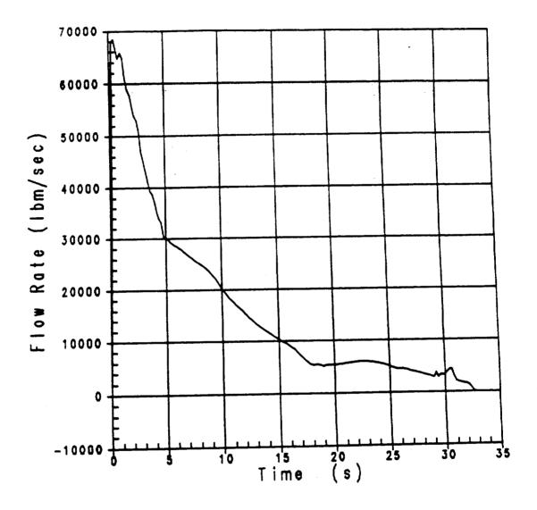
Figure 3.1-15 Break Flow During Blowdown Uprating Analysis - RHR Crosstie Closed,  $F_q = 2.335$
