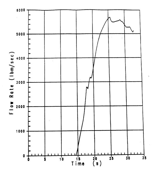
Figure 3.1-5 Accumulator Flow During Blowdown Uprating Analysis–RHR Crosstie Closed
