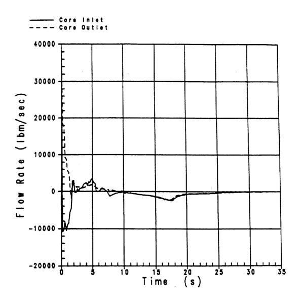
Figure 3.1-17 Core Flowrate Uprating Analysis - RHR Crosstie Closed,  $F_q = 2.335$
