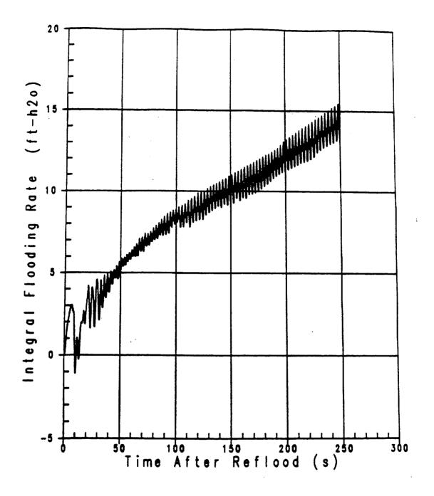
Figure 3.1-9 Integral of Core Inlet Flow Uprating Analysis–RHR Crosstie Closed
