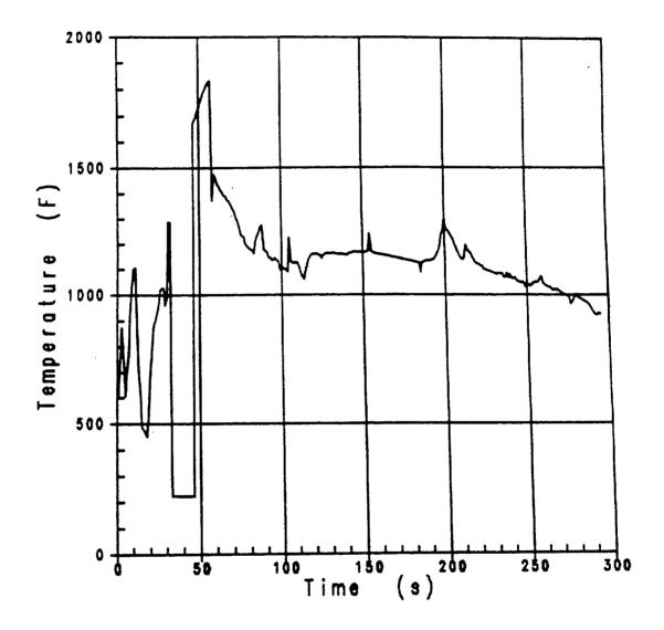
Figure 3.1-25 Vapor Temperature Uprating Analysis - RHR Crosstie Closed,  $F_q = 2.335$
