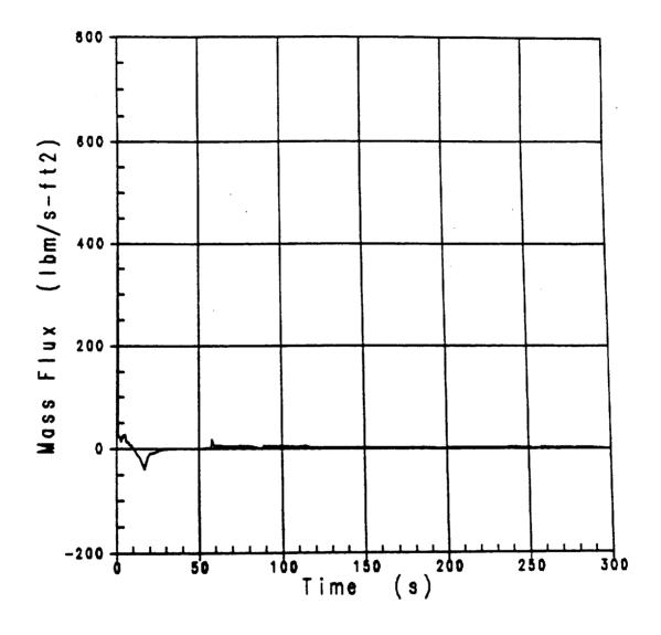
Figure 3.1-23 Mass Flux at Peak Temperature Elevation Uprating Analysis - RHR Crosstie Closed,  $F_q = 2.335$
