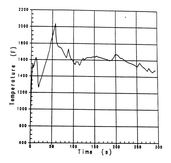
Figure 3.1-26 Fuel Rod Peak Clad Temperature Uprating Analysis - RHR Crosstie Closed, F<sub>q</sub> = 2.335
