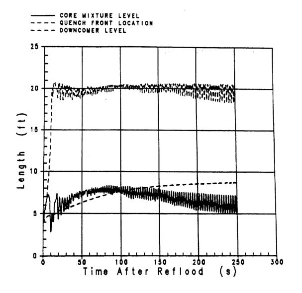
Figure 3.1-19 Vessel Liquid Levels During Reflood Uprating Analysis - RHR Crosstie Closed,  $F_a = 2.335$
