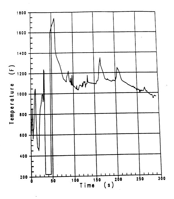
Figure 3.11-12 Vapor Temperature Uprating Analysis–RHR Crosstie Closed
