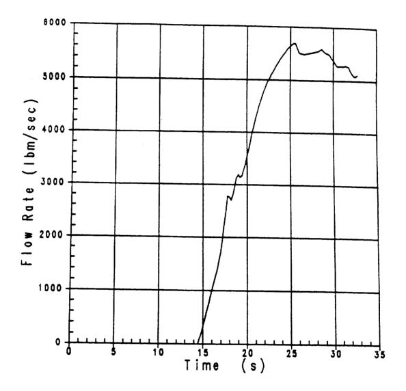
Figure 3.1-18 Accumulator Flow During Blowdown Uprating Analysis - RHR Crosstie Closed,  $F_{q} = 2.335$
