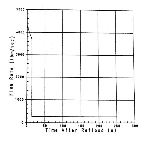
Figure 3.1-21 Accumulator and SI Flow During Reflood Uprating Analysis - RHR Crosstie Closed,  $F_q = 2.335$
