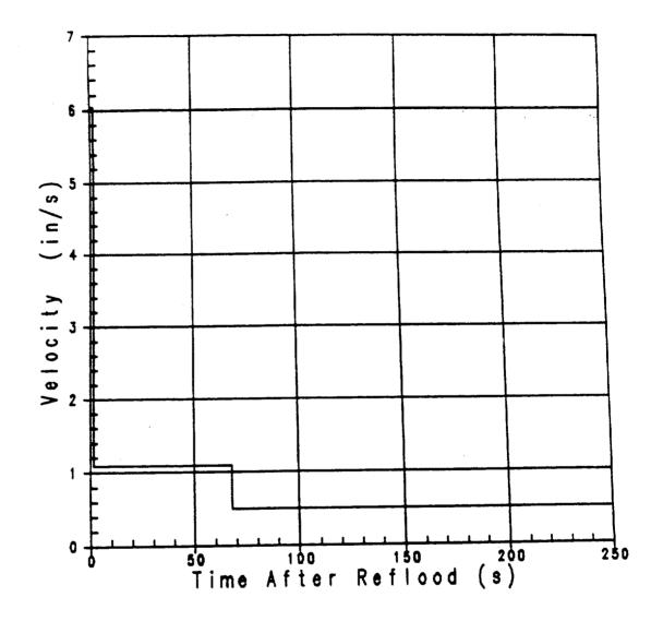
Figure 3.1-20 Core Inlet Flow During Reflood Uprating Analysis - RHR Crosstie Closed, F<sub>o</sub> = 2.335
