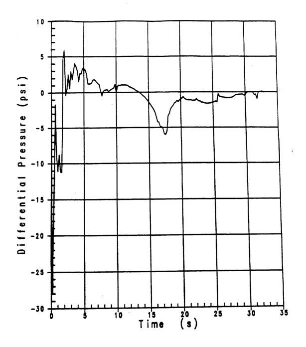
Figure 3.1-3 Core Pressure Drop Uprating Analysis–RHR Crosstie Closed
