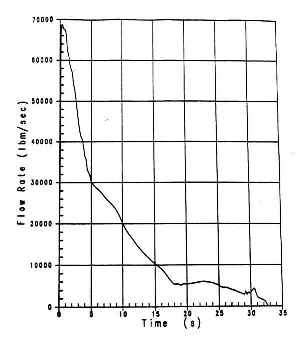
Figure 3.1-2 Break Flow During Blowdown Uprating Analysis–RHR Crosstie Closed
