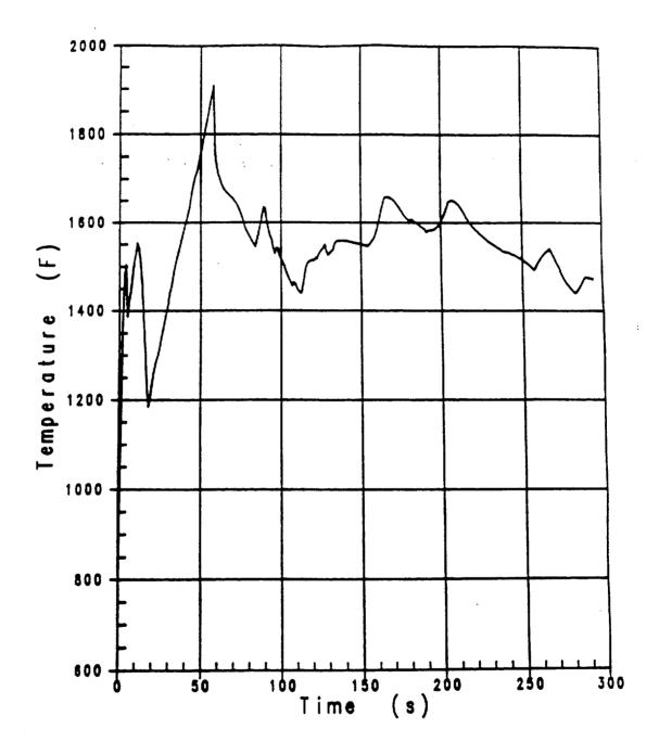
Figure 3.1-13 Fuel Rod Peak Clad Temperature Uprating Analysis–RHR Crosstie Closed
