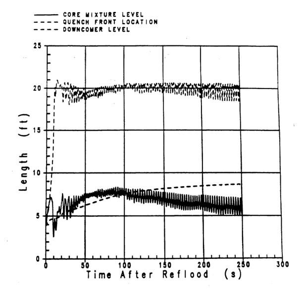
Figure 3.1-6 Vessel Liquid Levels During Reflood Uprating Analysis--RHR Crosstie Closed
