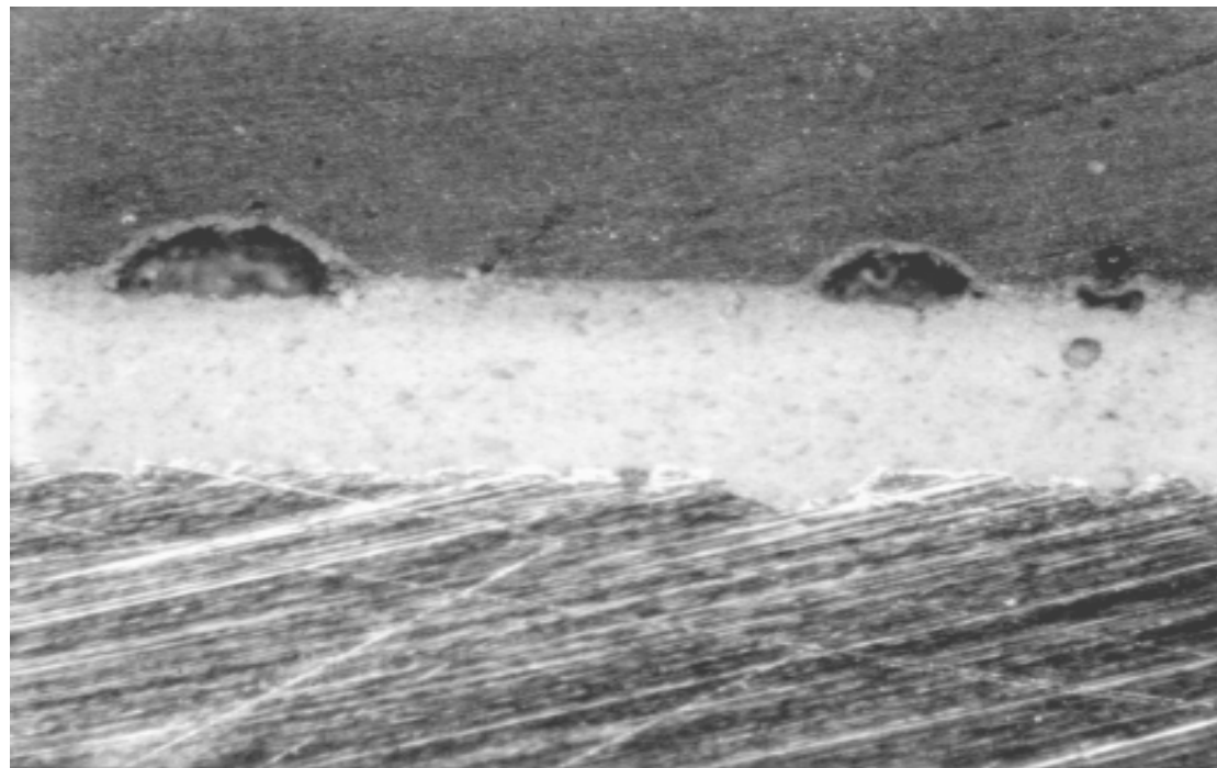
Aged Epoxy Polyamide (System 5) with blisters
