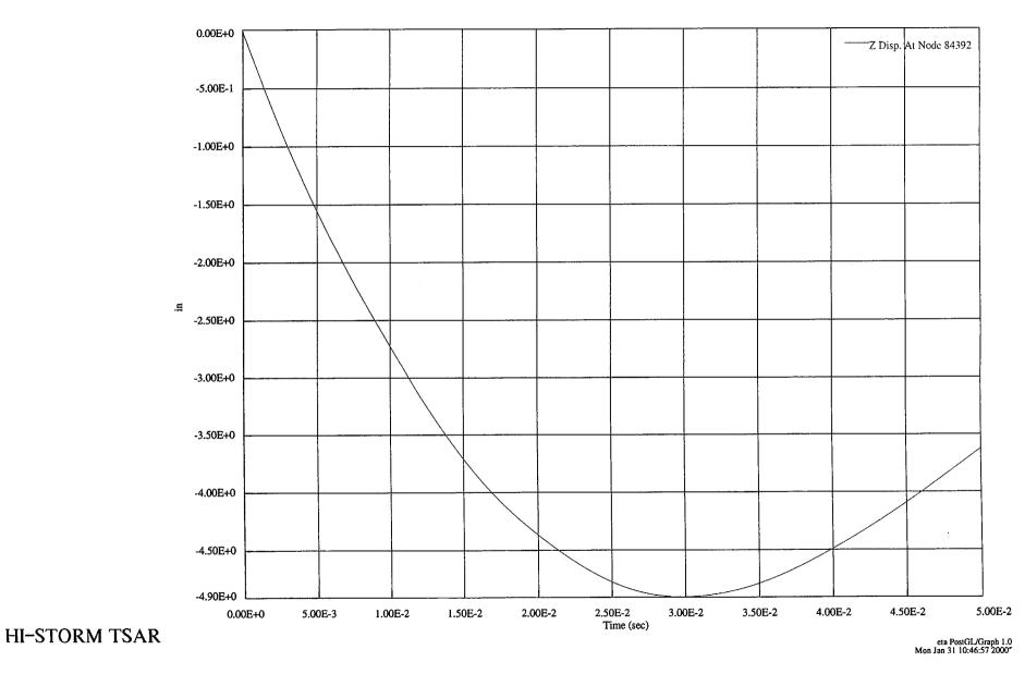
FIG. 3.A.20 Tipover Scenario: Channel A2 Displacement Time History
