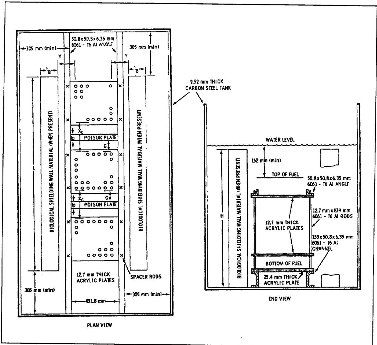
Figure 6.1 PNL Critical Experiment Layout (Reference 3)
