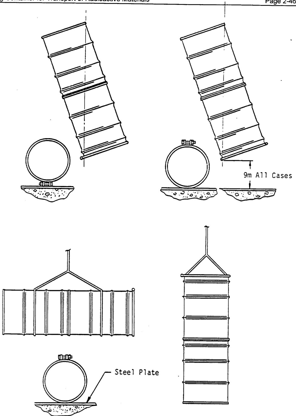
Fig. 2.9 9m (30 ft) Drop Test Orientations 10 CFR 71.73(c)(1)
