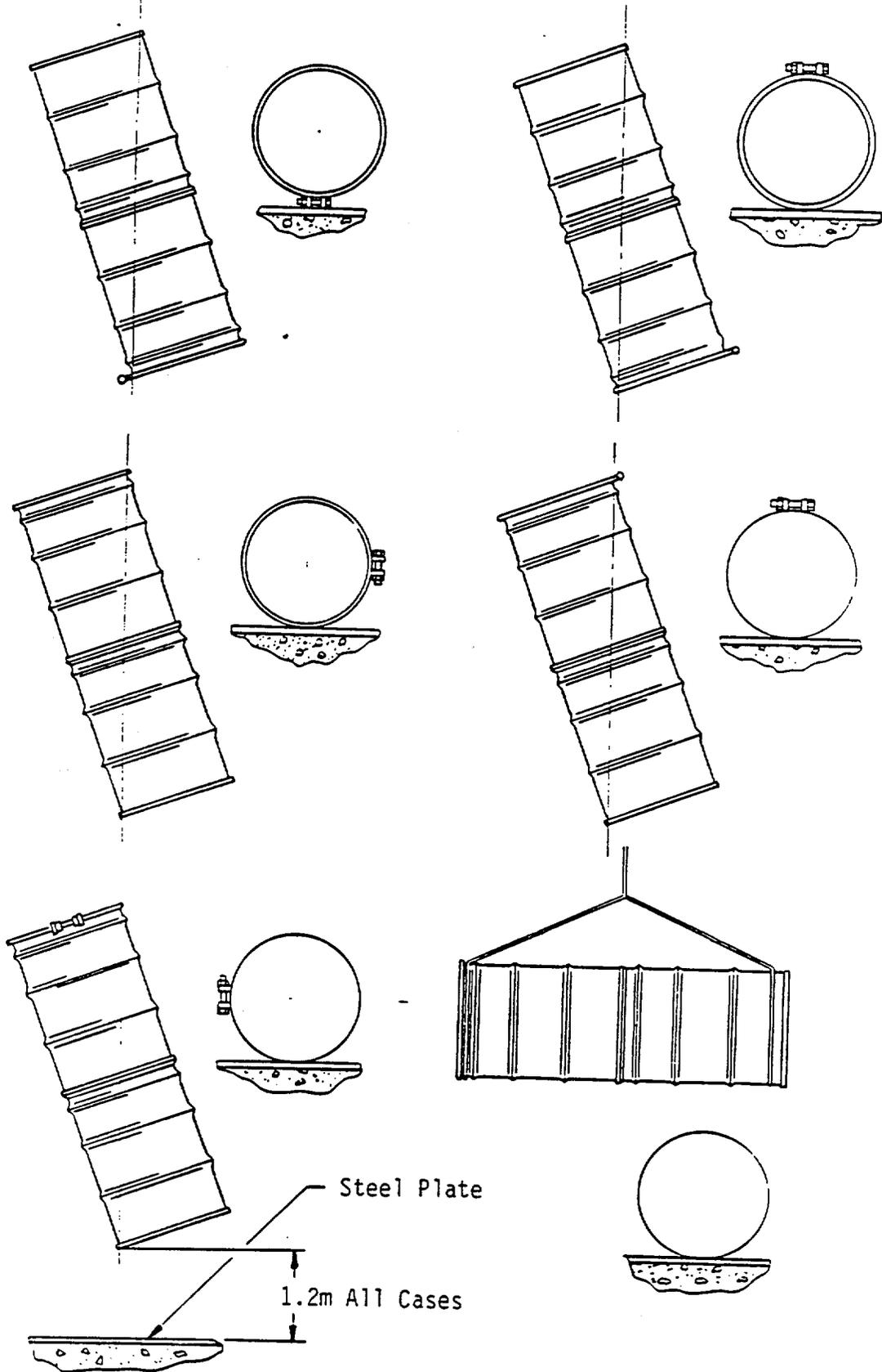
Fig. 2.5.2 1.2m (4 ft.) Drop Tests 10 CFR 71.71(c)(7)
