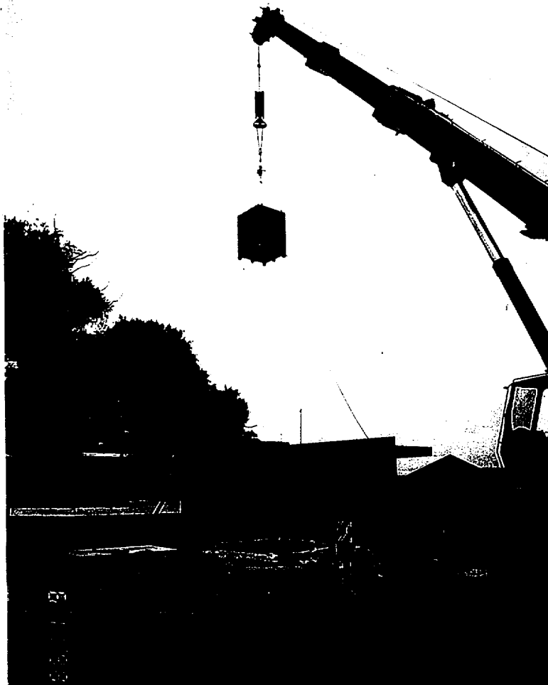
2.10.4p-8 Eco-Pak® OP Transport Unit - 30 Foot Free Drop onto Bottom
