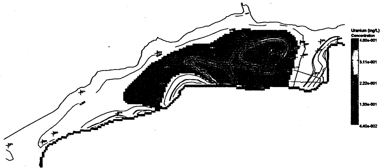
Figure 33. Predicted Uranium Concentrations in the Ground Water at the New Rifle Site at 10 Years — 100 Simulations
