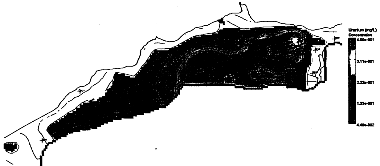
Figure 32. Initial Uranium Concentration in the Ground Water at the New Rifle Site Measured in July 1998
