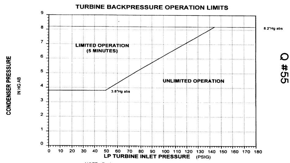
NOTE: Backpressure upper limit of <u>8.2"Hg abs</u> selected based on the Main Turbine Low Vacuum Trip of 21.5" @ barometric pressure of 29.7"Hg (see page two for x and y coordinate data points)
