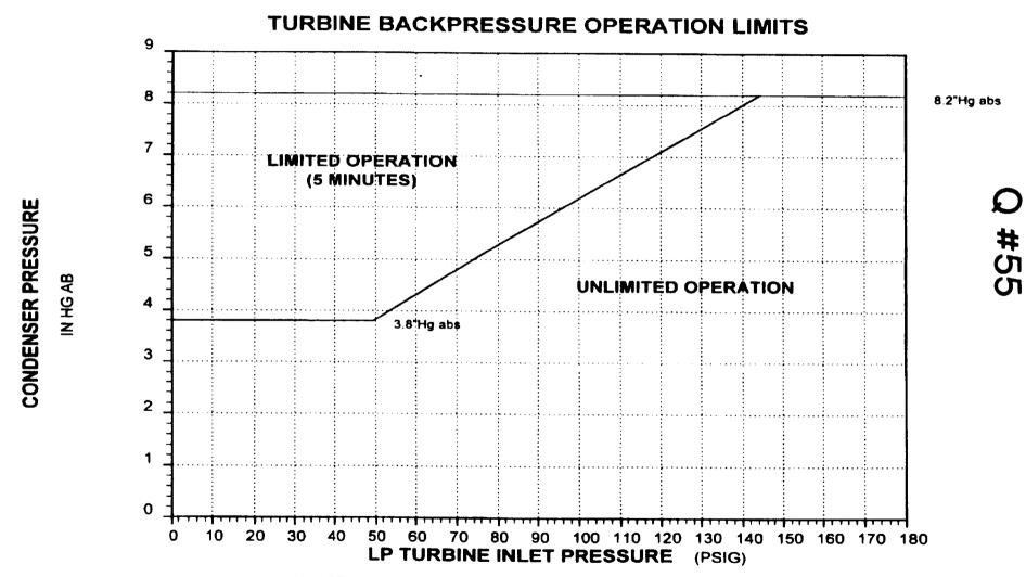
NOTE: Backpressure upper limit of <u>8.2"Hg abs</u> selected based on the Main Turbine Low Vacuum Trip of 21.5" @ barometric pressure of 29.7"Hg (see page two for x and y coordinate data points)
