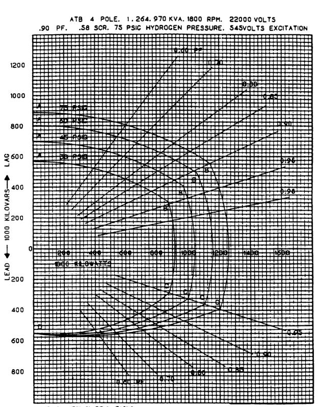
CURVE AB LIMITED BY FIELD HEATING CURVE BC LIMITED BY ARMATURE HEATING
