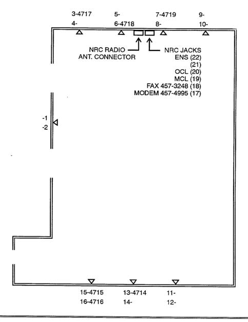
NOTE: Plug radios into their respective jacks (NRC supplies the radios).
